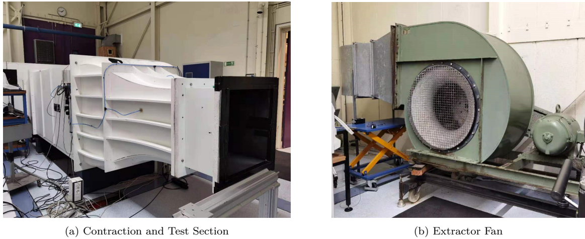
Figure 4.1: The W-Tunnel, both images reproduced from TU Delft Aerodynamics Experimental Wiki [2]
