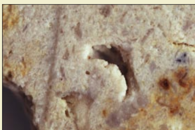
If we zoom in on the sectional plane, several small cavities can be seen which give the impression that the stone might have been cast, since such a process could easily trap air bubbles inside the material.
