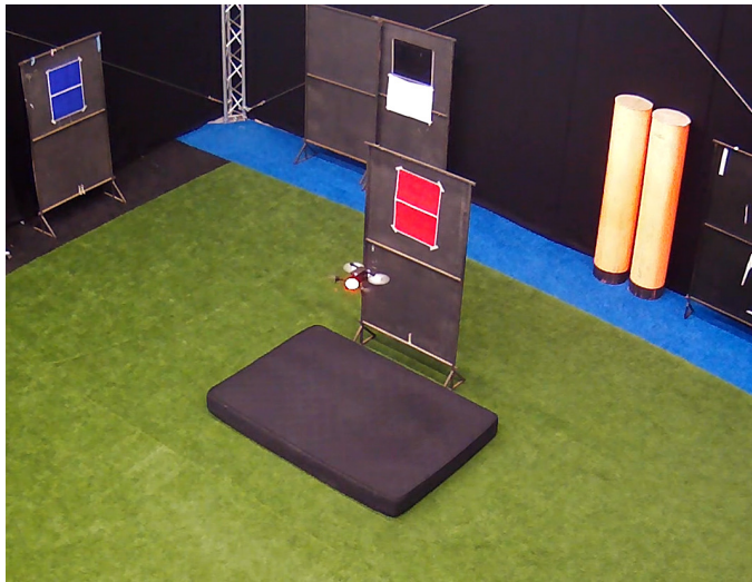
Figure 2.19: Parrot Bebop 2 with SLAMDunk stopping in front of an obstacle using SGBM and OptiTrack. (March 2018.)
