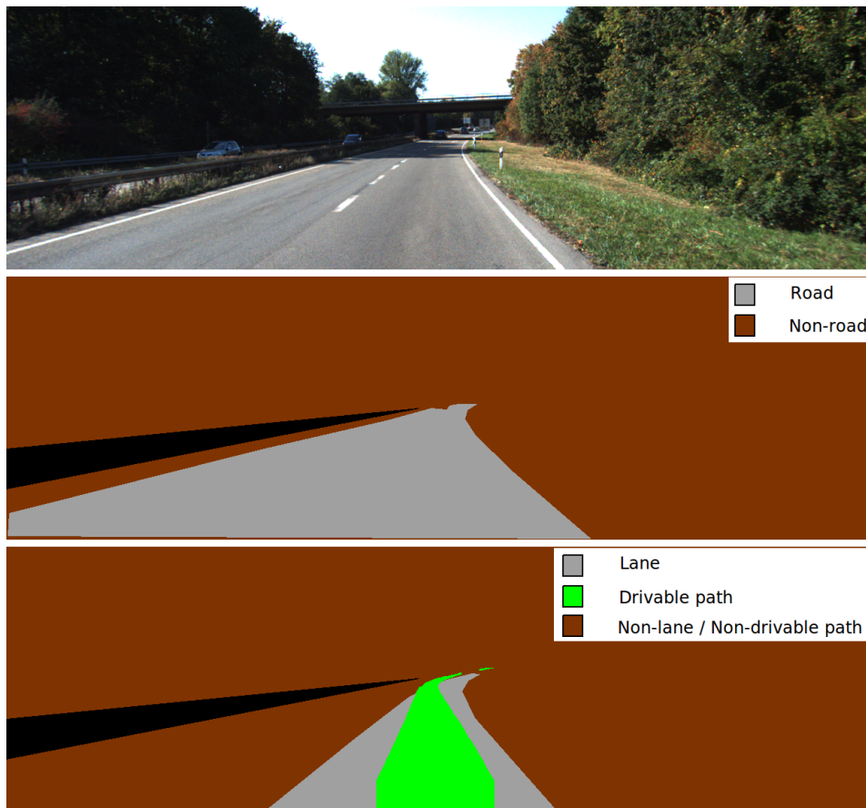
Figure 2.11: Visualisation of the difference between road segmentation (middle; grey area) and lane segmentation (lower; grey area) and drivable path (lower; green area). NOTE: the lane change of the drivable path can clearly be seen in the lower image.
