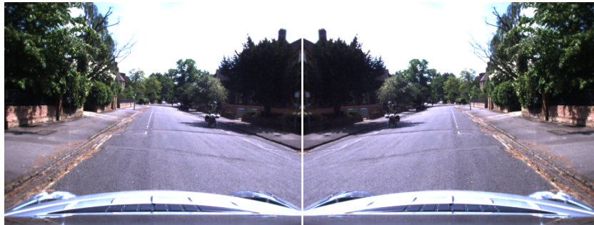
Figure 3.8: Original image of the RobotCar training set (left), after the flipping procedure (right).
