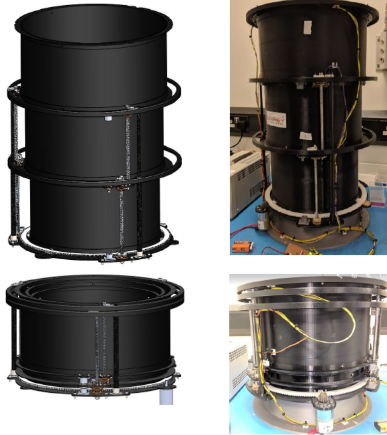
Figure 8.10: Surrey Satellite Technologies Limited their telescopic optical barrel in deployed and stowed configuration in Solidworks (left) and breadboard model (right) [13]
