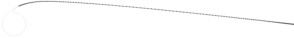
(a) Tanh node distribution along the upper and lower canopy surface.
