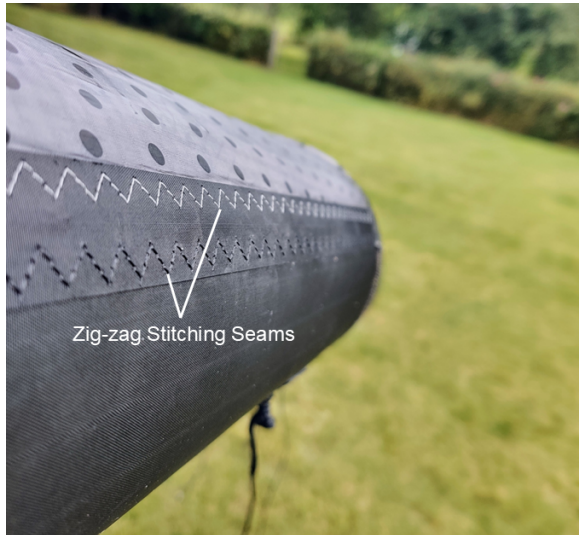
Figure 2.8: Stitching seams with canopy overlay near the upper surface of the LE tube.
