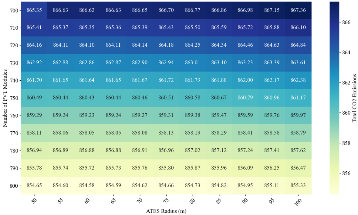
Figure 58: Total CO 2 Emissions for Different PVT Modules and ATES Radii
