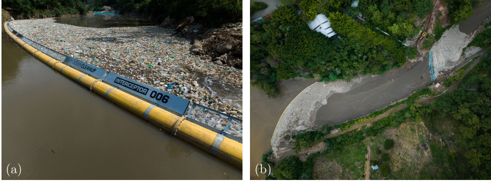
Figure 2.1: Accumulation of plastic debris at waste-collection devices, creating the so-called carpet . (a) Plastic debris captured by the floating boom, looking at upstream direction. (b) Aerial view of the carpet formations upstream of the waste-collection device. Photo Credit: The Ocean Cleanup.
