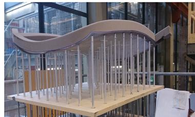
Figure 4.8: Deflection of the elastic layer on 120mm grid distance
