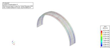
Figure C.7: Reinforcement stress distribution SXX due to prestressing steel loads - DIANA10.2
