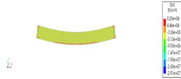
Figure 6.16: Total concrete stresses (P+SW+F) SXX - F.C.
