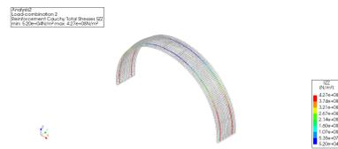
Figure C.8: Reinforcement stress distribution SZZ due to prestressing steel loads - DIANA10.2
