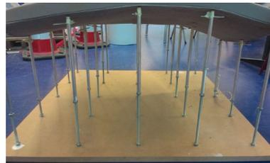
Figure 4.6: Deflection of the elastic layer on 240mm grid distance
