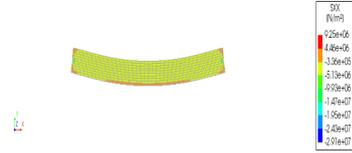
Figure 6.16: Total concrete stresses (P+SW+F) SXX - F.C.
