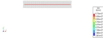
Figure A.57: Prestressing steel stresses SXX - LC4
