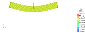
Figure 6.31: Concrete stresses SXX - L.S. 14
