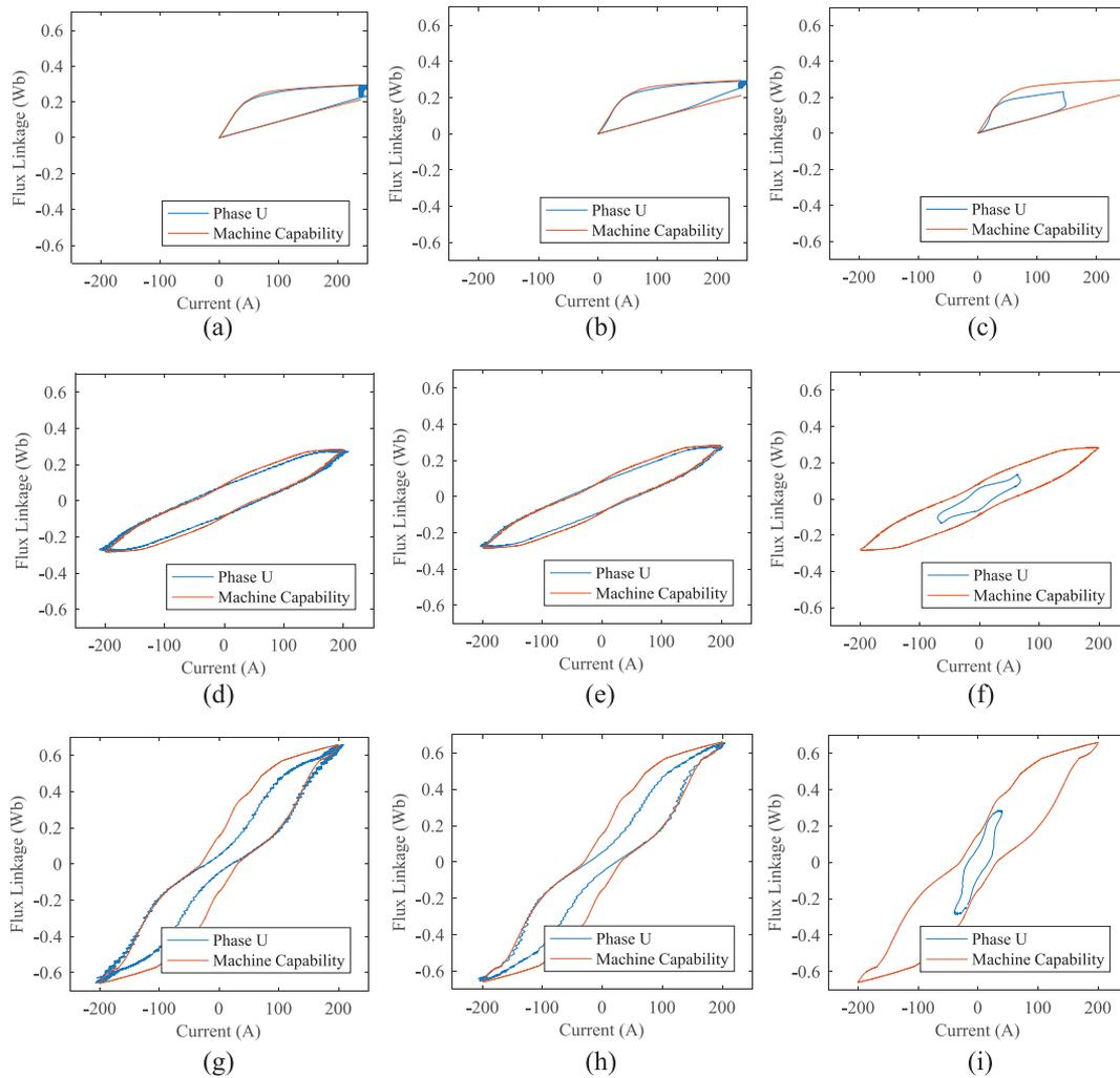
Fig. 11. Phase flux linkage-current curves of each motor at different speeds: (a) CSRM at 1000 rpm (b) CSRM at 2000 rpm (c) CSRM at 5000 rpm. (d) MCSRM at 1000 rpm (e) MCSRM at 2000 rpm (f) MCSRM at 5000 rpm. (g) TWSRM at 1000 rpm (h) TWSRM at 2000 rpm (i) TWSRM at 5000 rpm.
