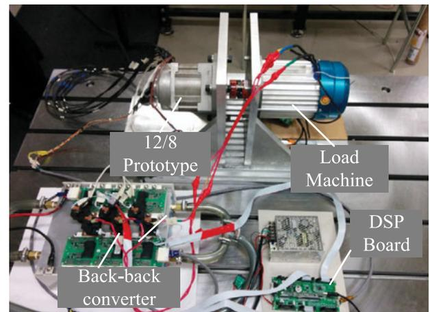
Fig. 12. Experimental setup based on the 12/8 MCSRM prototype.
