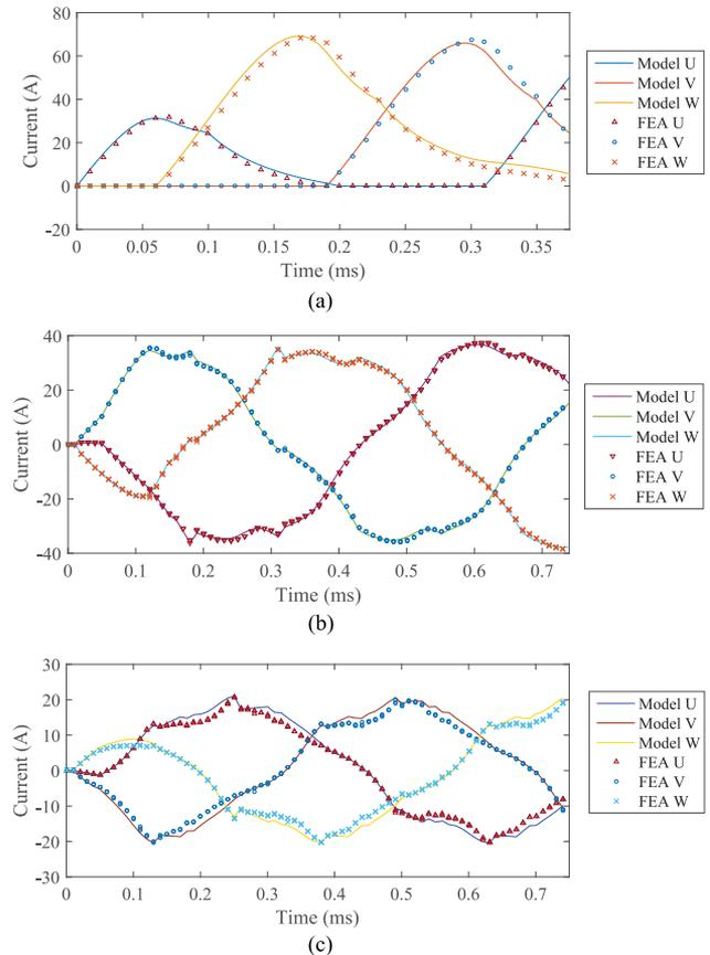
Fig. 10. Current waveforms comparison between dynamic models and FEA at 10000 rpm (a) CSRSM, (b) MCSRM and (c) TWSRM.
