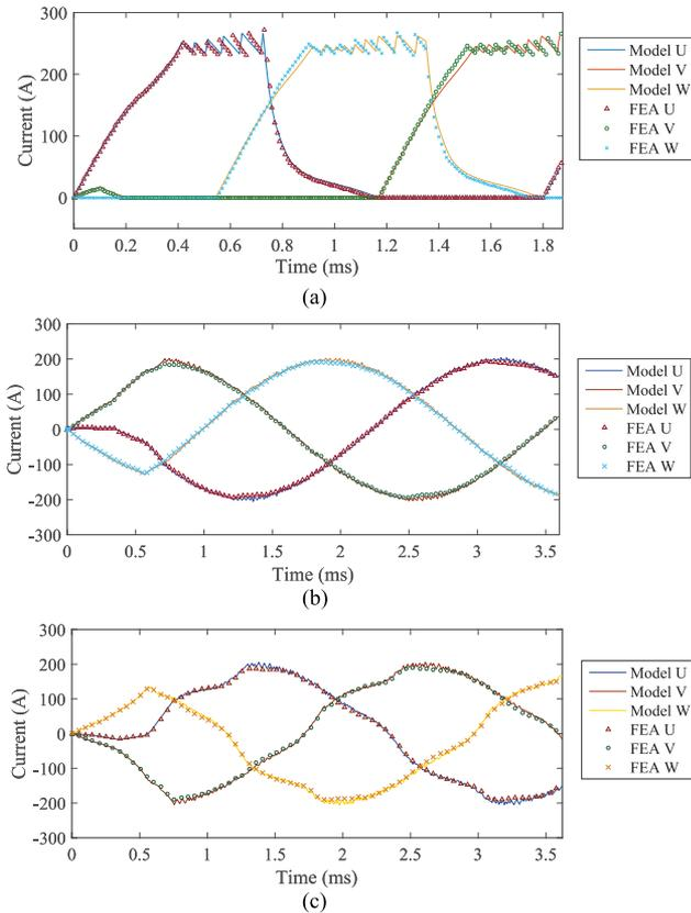
Fig. 9. Current waveforms comparison between dynamic models and FEA at 2000 rpm (a) CSRSM, (b) MCSRM and (c) TWSRM.
