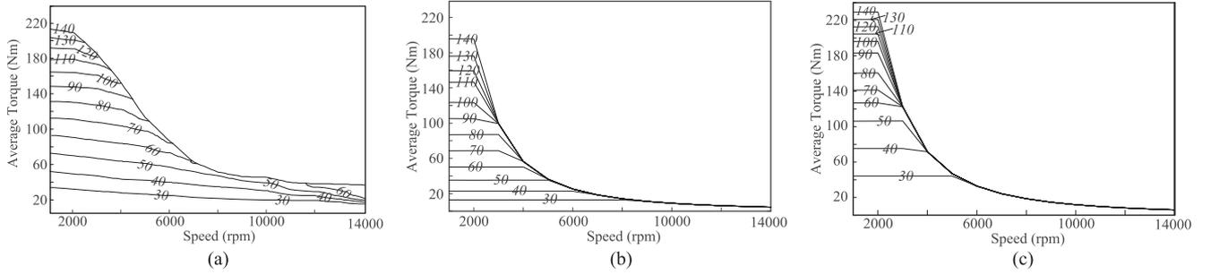
Fig. 8. Torque-speed curve of the motors under different current constraints: (a) CSRM, (b) MCSRM and (c) TWSRM.
