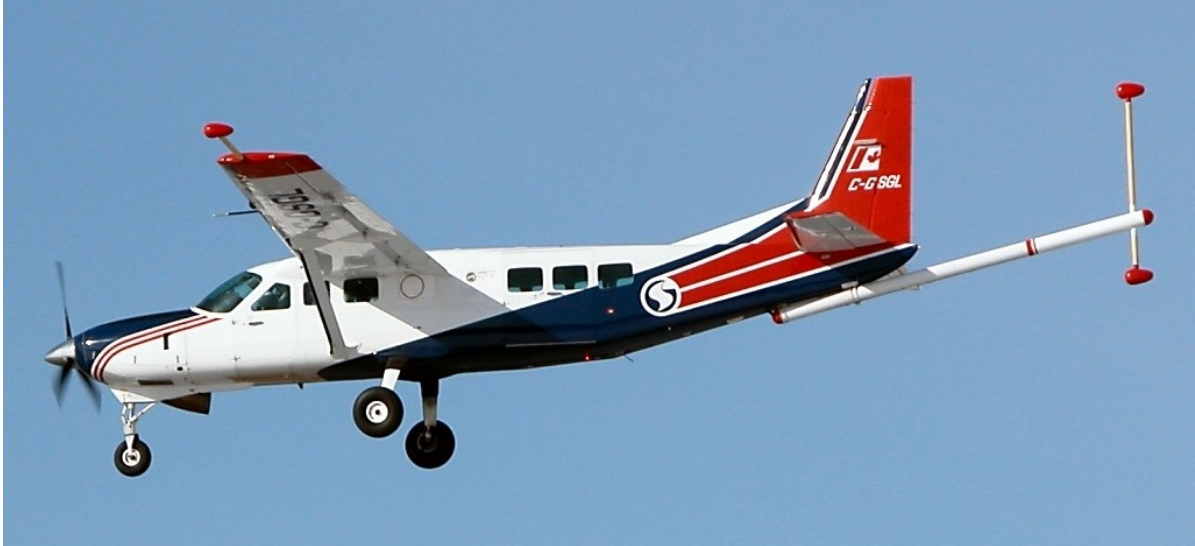
Figure 1.1: Geosurvey aircraft similar to the one used by Canciani. Note the tail-stinger at the rear of the aircraft. At the tip of the tail-stinger there are magnetometers. Source: [19].
