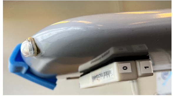
Figure 3.2: Close-up of the Mugin fixed-wing drone right side wing tip. The MicroSAM OPM magnetometer is labelled with '0' and the VMR vector magnetometer is labelled with '1'.
