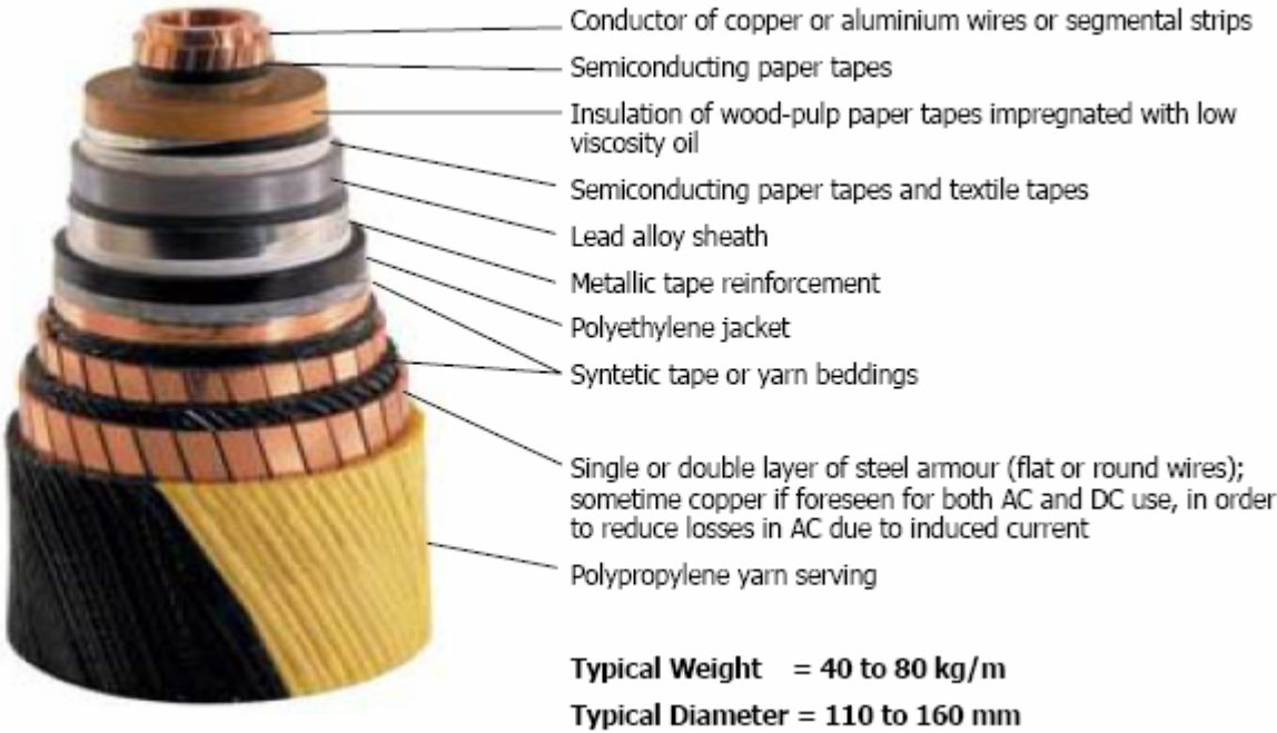
Figure 3.5 The self contained fluid-filled power cable [67]
