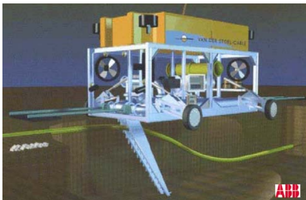
Figure 3.15 The hydraulic jet plough/ towed jetting vehicle [75]
