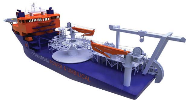
Figure 3.13 The cable layer [92]
