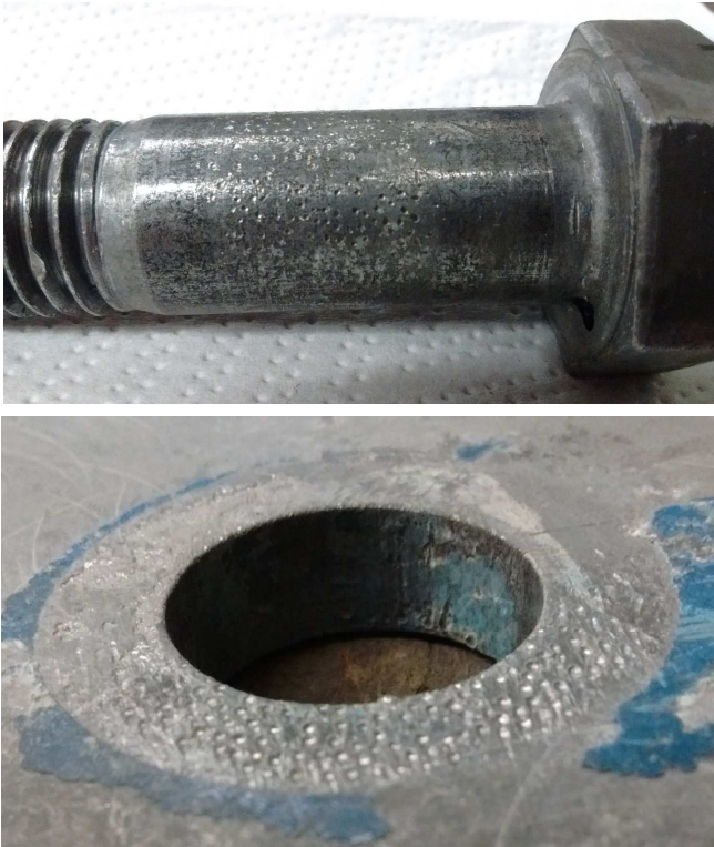
Figure 109 - Indentation of shot in bolt (top) and plate surface (bottom)
