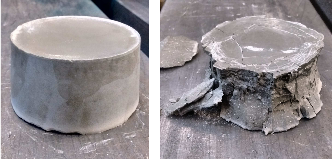
Figure 67 - Small-scale grout sample used to determine the compressive strength, before (left) and after (right) loading in a compression machine.
