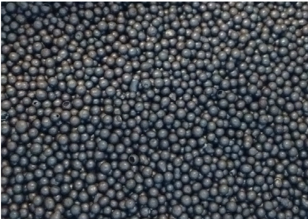
Figure 96 - Steel shot of size class S330 (nominal diameter 1 mm) as used in the experiments
