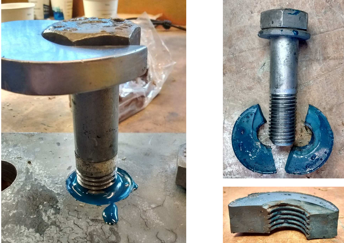
Figure 57 – Left: Unscrewing a bolt from resin infill using a wrench. Right (top): disassembled components. Right (bottom): cross section of resin infill showing the bolt threads cast into the resin.
