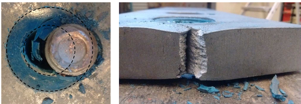
Figure 70 - Condition of centre plate with \varnothing_{centre} = 36 mm after being loaded to ultimate failure
