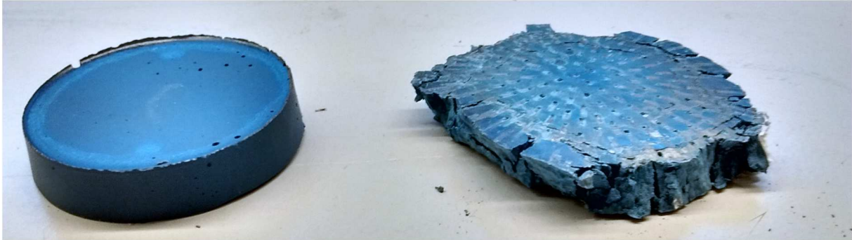
Figure 63 - Small-scale resin sample used to determine the compressive strength, before (left) and after (right) loading in a compression machine.
