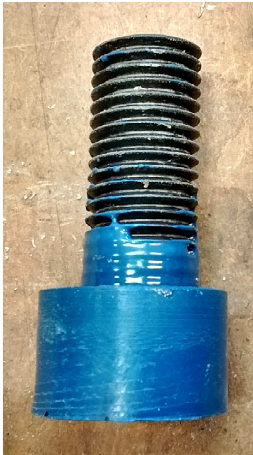
Figure 56 - Left: threaded end including resin released from a mould treated with a wax-based release agent. Right: Formation of threads in the resin: due to application of a waxy release agent the threaded end could be removed by unscrewing
