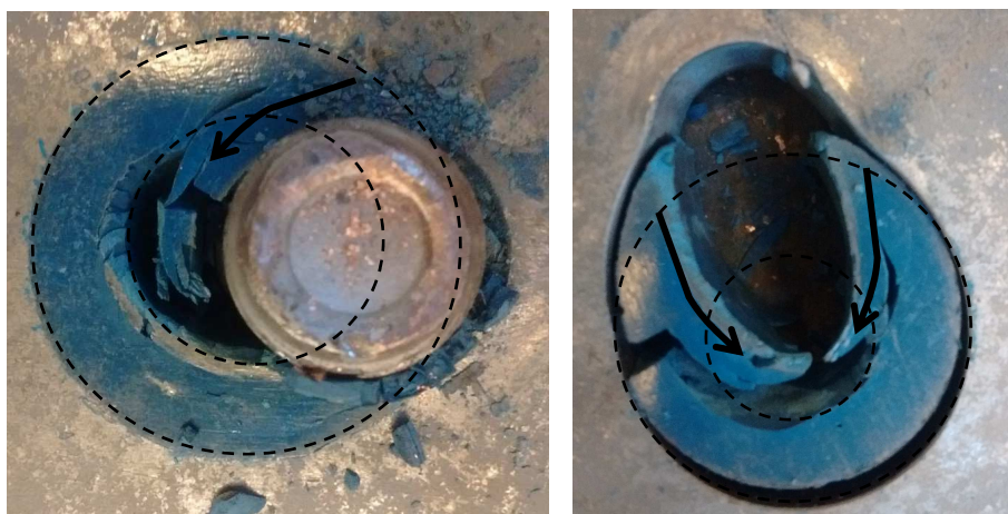
Figure 124 - Rigid body movement (sliding) of parts of resin within centre plate
