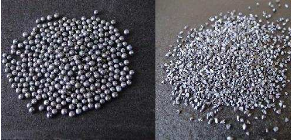
Figure 114- Particles with different geometrical characteristics. Left: shot (spherical), right: grit (irregularly shaped) (Shanghai Bosun Abrasive Co., Ltd.)
