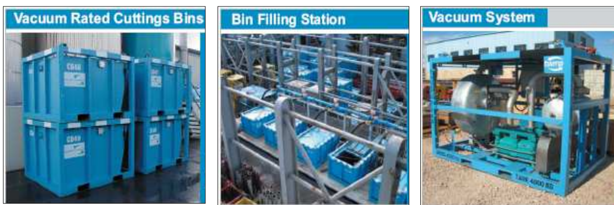
Figure 4.1: Illustration: TWMA (Norway) Integrated Drilling Waste Management system.
