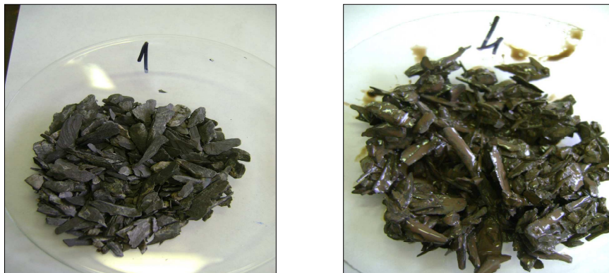
Figure 9.2: Drill cuttings (left) and drilling mud with cuttings (right) from shale shaker
