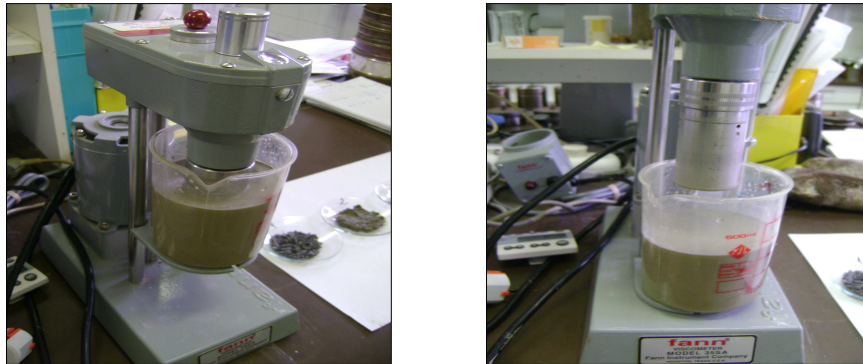
Figure 9.5: Viscosity measurement of samples using Fann Viscometer
