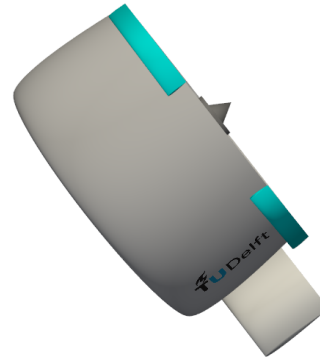
Figure 6.31: Conceptual illustration of the proposed control vane configuration used in the DUUC V0.9.
