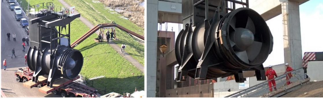
**Figure 2.4:** An example of a pump that is installed at the pumping station of IJmuiden [24, 25]
