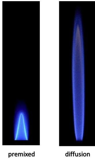
(a) Luminous images of the premixed and diffusion flames at the same air and fuel flow rates; source [42] (b) NOx emissions for diffusion ( PB = 0\% ), premixed ( PB = 100\% ) and partially premixed ( PB = 92\% ) flames vs. normalized Air/Fuel ratio \lambda = \frac{1}{\phi} ; source [19]
