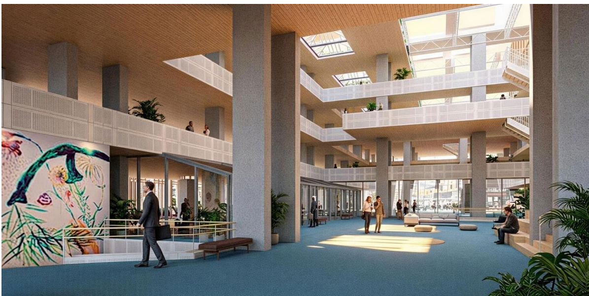
Figure 5: Example of how fixed attributes are considered during the design process. The wall painting (left) is existing and spans from the ground floor to the basement. This is preserved and used to guide people to the reading room downstairs. The structure of the atriums is also preserved and opened up to emphasize this. Also, the aluminium interior cladding is brought back.
