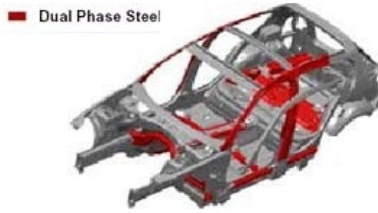
Figure 1.2: Application of Dual Phase steel in the automobile chassis (SalzgitterFlachstahl [2013])
