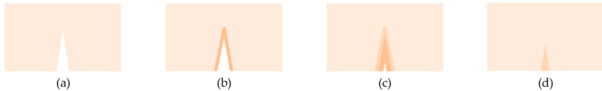
Figure 1. The basic principle of crack healing in asphalt pavement: (a) a crack generated in asphalt mastic; (b) the ‘mobile phase’ induced at the crack face; (c) closure of the crack by the ‘mobile phase’ and (d) immobilisation after healing (Hager et al., 2010).
