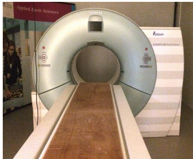
Figure 14: Siemens SOMATOM Definition macro-CT scanner used for CT scans on frozen samples
