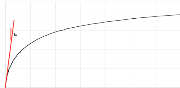
Figure 24: Schematic of stiffness calculation from strength vs. stress graphs
