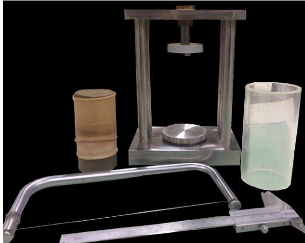
Figure 11: Sample cutting equipment (clockwise from top left): cut sample with membrane, cutting frame, plastic cylinder for installing membrane, callipers, wire cutter
