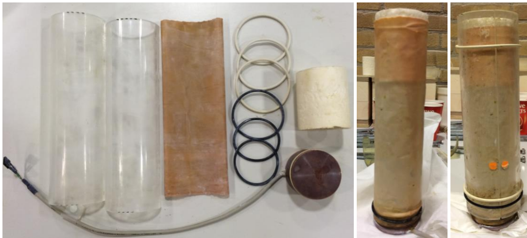
Figure 8: LEFT: Disassembled sample casing; CENTRE: Assembled sample without Perspex cylinder; RIGHT: Assembled sample in Perspex cylinder
