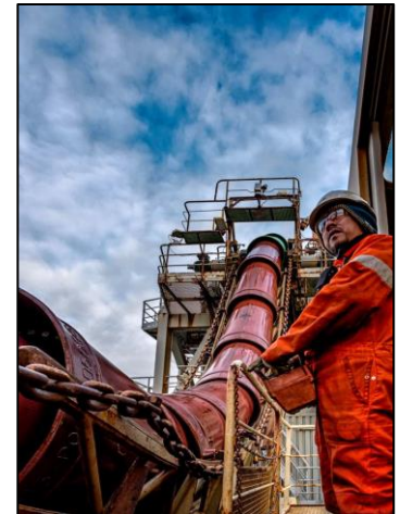
Figure 3.1 String of buckets of flexible fallpipe on board of vessel Nordnes. Image: Van Oord (2021).
