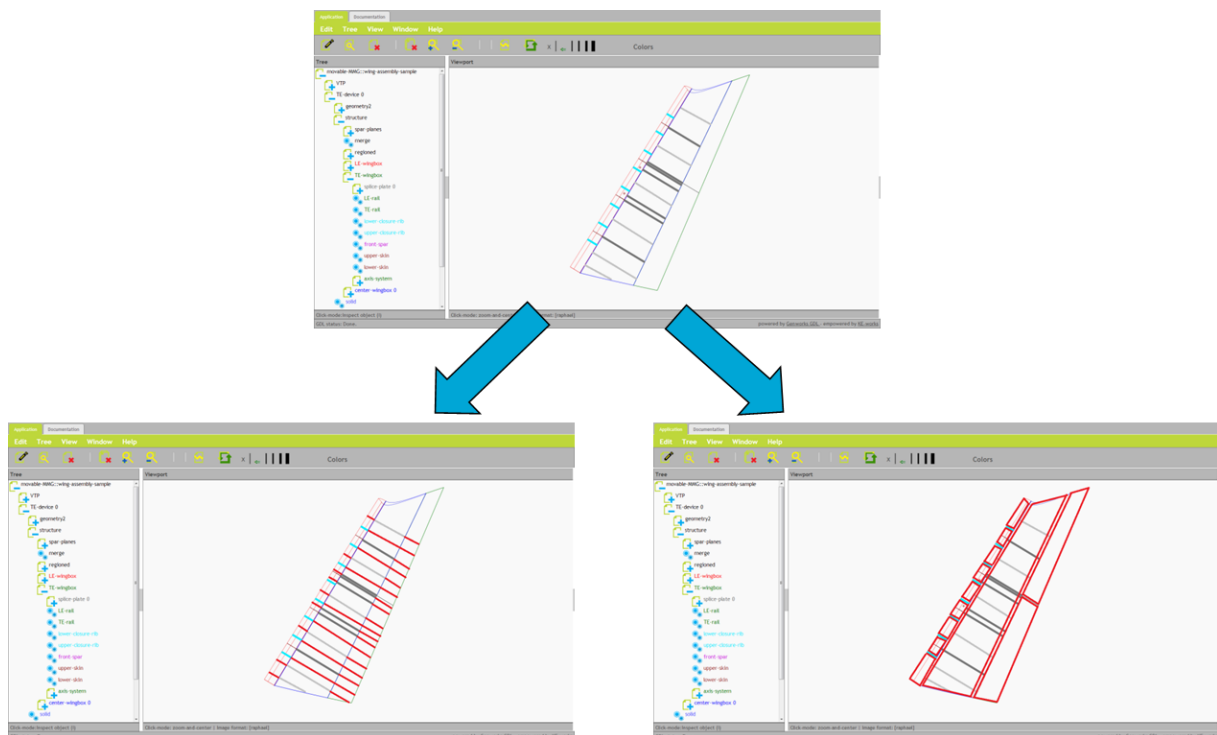
Figure 7: two subdivision steps are required to derive the appropriate perspective for both FEM analysis (left) and manufacturing / weight analyses (right). The red boundaries highlight the domain-specific segmentation.
