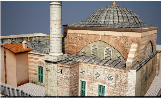
Figure 6. The LOD 2 Representation of a Mosque Generated based on Terrestrial Laser Scanning Data
