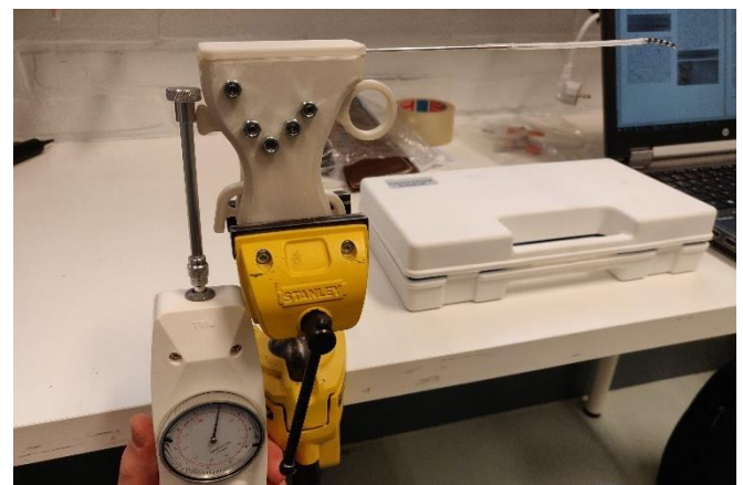
Figure 29. The setup of the first preparation step experiment consisted of a push pull force gauge (white), a bench vise (yellow), and a table.
