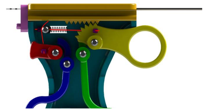
Figure 46. Redesign of the handle with a spring to allow lateral movement of the pulling cable axis, three cable locks (purple), and a Luer lock (pink) that is attached to the rear casing part (light blue). The Luer lock has a proximal button to engage the lock. The radius adjustment button (red) is shortened. An extra pulling cable (red, right) is added between the bending trigger and the axis of the other pulling cable (red, left).
