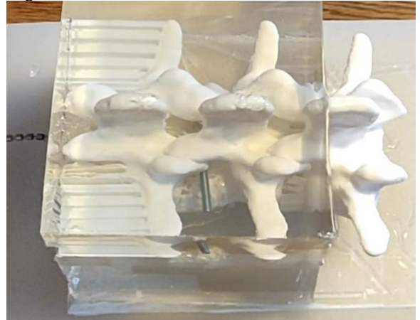
Figure 32. The complete procedure experiment setup consisted of three L3 spinal vertebrae 3D-printed on top of each other surrounded by gelatin. The steerable tip was inserted into the spinal cord lumen from the bottom of the vertebrae and aimed to surround the M3 bolt that mimics the DRG. The vertebrae were positioned on a plastic cutting board on top of a table.
