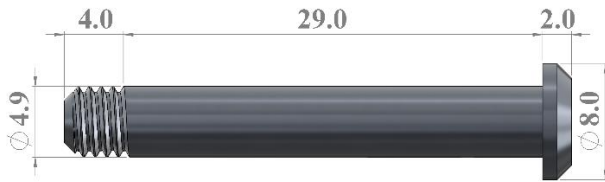
Figure 22. The machined screws with dimensions in mm.
