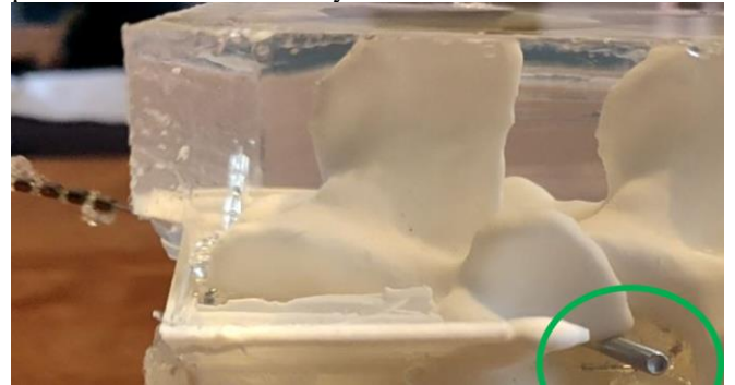
Figure 43. The implanted electrode lead around an M3 bolt (green circle) that mimicked a DRG in the intervertebral foramen of a 3D-printed vertebrae surrounded by gelatin.
