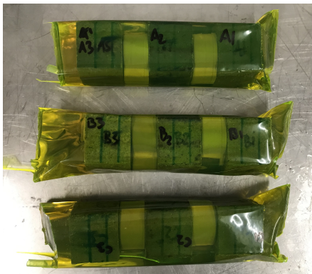
Figure 6.5: Specimens impregnated with epoxy ( Author's figure )
