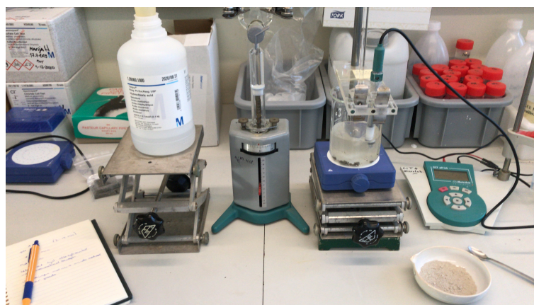
Figure 6.7: The titration set up for the buffer capacity test ( Author's figure )
