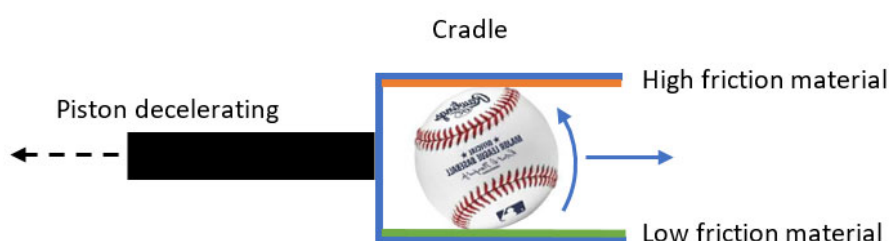
Figure 3. Schematic of the cradle attached to the pneumatic piston, showing spin imparted to the baseball as the piston decelerates.
