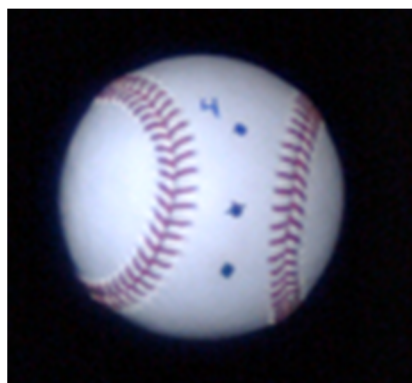
Figure 4. Image of tracking dots on baseball that were used to measure spin.
