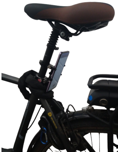
Figure 2.2: Smartphone rigidly mounted at the back of the seat post.
