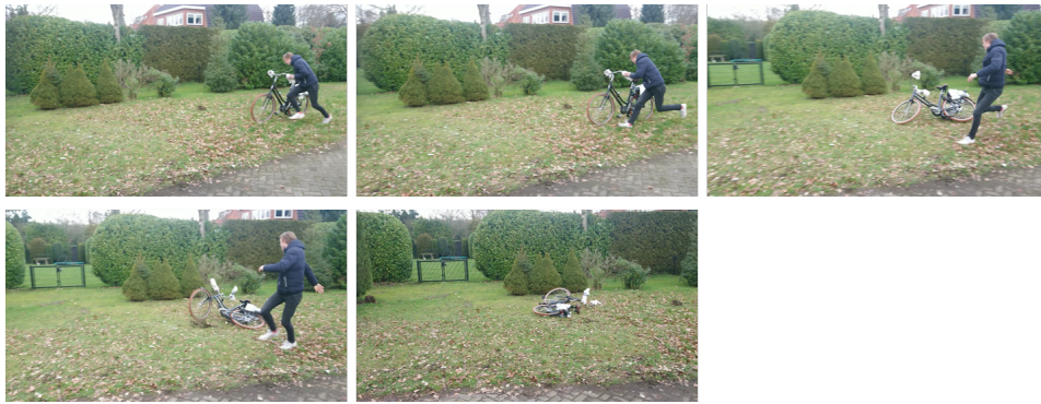
Figure 2.4: Push fall (P4), a simulated fall where the bicycle is pushed forward and then to the side at 22 km/h . See also appendix C.3.
