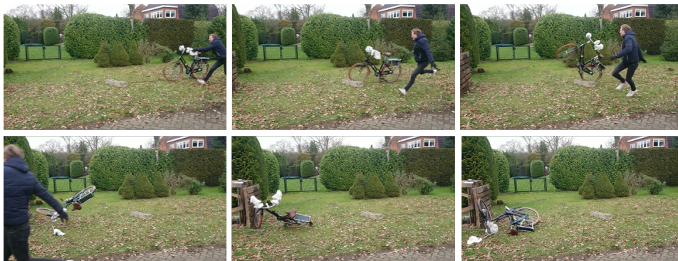
Figure 2.5: Collision into a curb (S4), a simulated collision where the bicycle is pushed into a curb at 45° at 22 km/h . See also appendix C.4.
