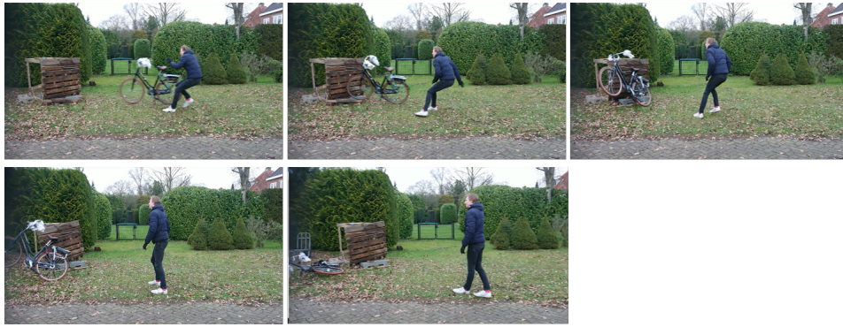
Figure 2.7: Collision into a wall (H4), a simulated collision where the bicycle is pushed into a wall at 45^\circ at 22 \text{ km/h} . See also appendix C.6.
