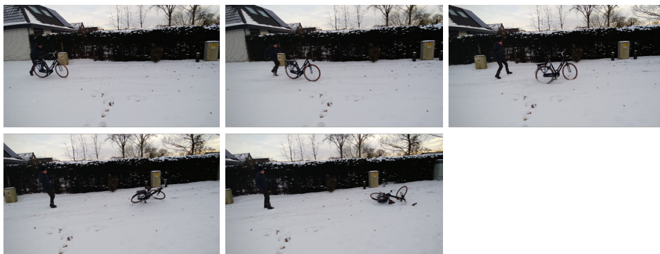
Figure 2.9: Skid-Fall (D10), a simulated skid where the bicycle is pushed forward and then to the side at 20 \text{ km/h} on a snowy road. See also appendix C.8.
