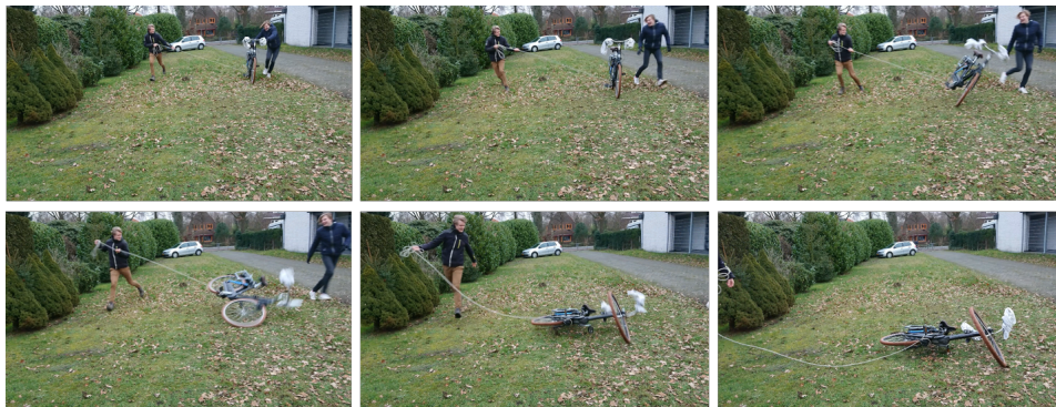
Figure 2.8: Skid (Q4), a simulated skid where the bicycle is pushed and let go at 22 \text{ km/h} . When the bicycle is let go, the bottom of the frame is pulled to the right with a rope. See also appendix C.7.
