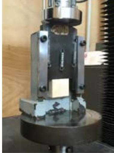
**Fig. 2** Block shear testing device
