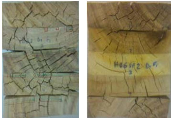
Figure 5: Delamination specimens after 3<sup>rd</sup> test cycle (Method A): BG3-D1 specimen (left) and HBGBP2-D1 specimen (right)
