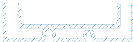
Figure B5.6 Crosssections of a kiss-off and an 'Almost' kiss-off rib (after Crawford, 1992)
