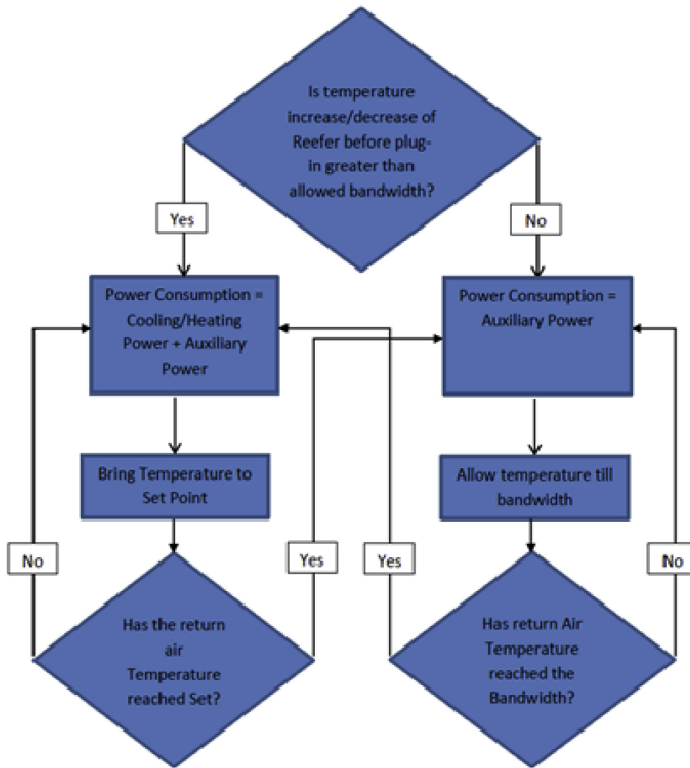
Fig. 6. Conceptual model for the power consumption of an individual reefer (Nafde, 2015).
