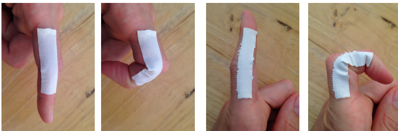
Figure 4-22 Bending of plaster causes bulges. Test is done with cotton tape (left) and gaffa tape (right).
