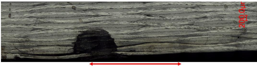
Figure 6.90: After 11,750 cycles, the meta-delamination has grown into a larger delamination. Note that the big spot is probably degraded matrix material which is expelled from the larger defect upon final cleaning of the polished surface.
