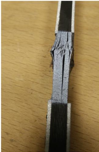
Figure 5.18: Aluminum sample 4. Broken in the middle under cyclic compressive loading.
