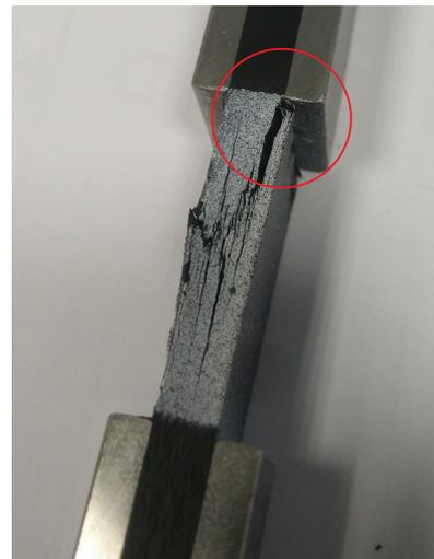
Figure 5.17: Steel sample 1. Fracture initiates in the stress concentration region for static loading.
