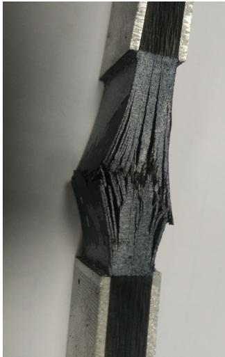
Figure 5.16: Aluminum sample 1. Broken in the middle under static loading.
