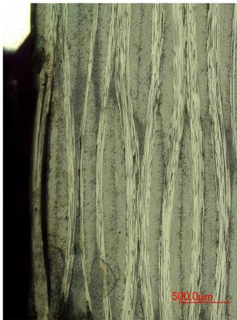
Figure 6.88: After 4,500 cycles, the sample showed a meta-delamination in the stress concentration region.
