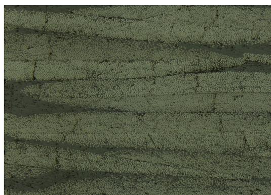
Figure 6.92: For a  $[\#(\pm 45)]_{24}$  laminate under T-C loading, many cracks can be observed
