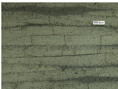
Figure 6.91: For a  $[\#(\pm 45)]_{24}$  laminate under C-C loading, cracks in bundles often combine through bundle debonding.
