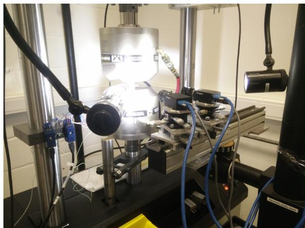
Figure 4.7: Camera set-up for 3D DIC
