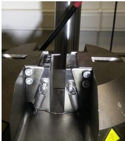
Figure 5.4: Hydraulic wedge clamps on the Instron test bench
