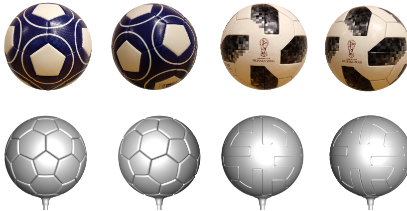
Figure 4.3: The footballs and orientations used, as seen in reality (top) and the CAD models showing the panels more clearly (bottom). Telstar: 0^\circ , 30^\circ . Telstar 18: 0^\circ , 17^\circ .
