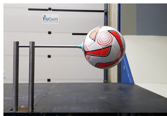
Figure 4.6: Second balance measurements setup showing the Telstar ball with sting from behind.
