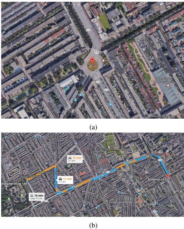
Figure 10. Wrong georeferencing of IFC models. (a) Provided position of the Rabarberstraat 144. (b) Distance comparison between the provided and the real positions. Images and map data taken from Google Maps.
