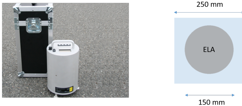
Figure 5.3: ELAtextur machine and consequent sampling dimension
