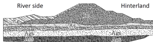
(a) The estimated soil pedophile of Yabe River levee at station 7.4km
