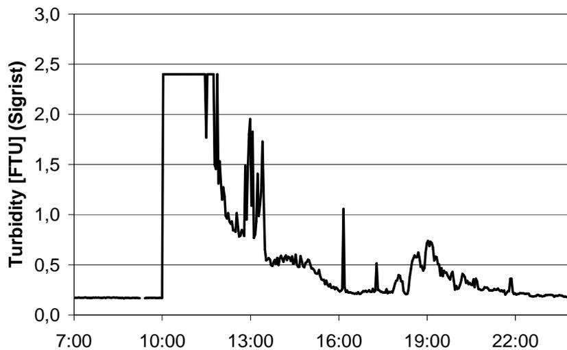
*Fig 2-16 Example of RPM, measured with Sigrist-equipment with maximum scale 2,4 FTU, indicating a high discoloration risk with a maximum score of 15. The increased velocity occurred from 10:00 to 10:15 and the effect is long measurable.*
