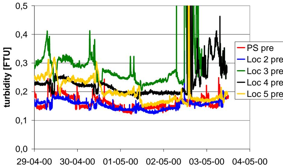
*Fig 5-17 Turbidity measurements during pre-cleaning period; on 2 May the RPM is determined*
