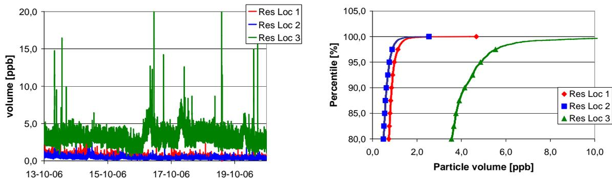
Fig 3-8 Calculated particle volumes in Research Area and cumulative frequency distribution during second measuring period
