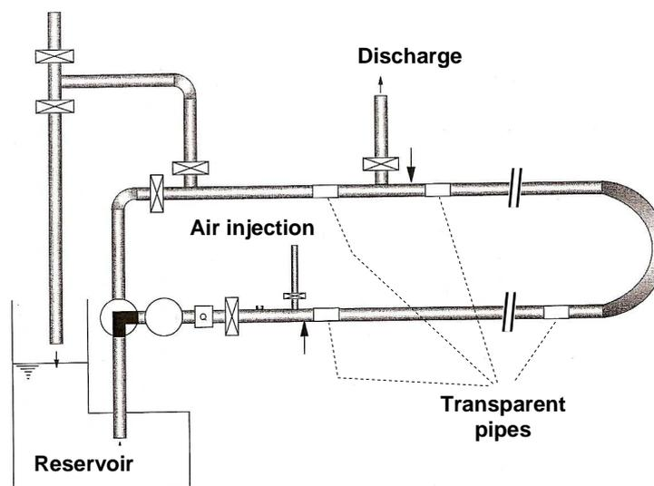
Fig 5-5 Experimental setup of water/air scouring test rig
