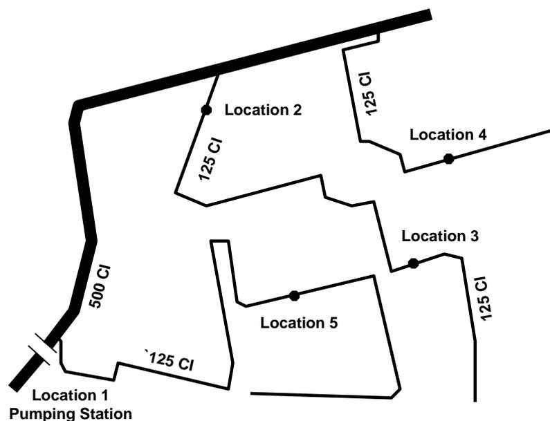
*Fig 5-16 Monitoring locations in cast iron network Tilburg*
