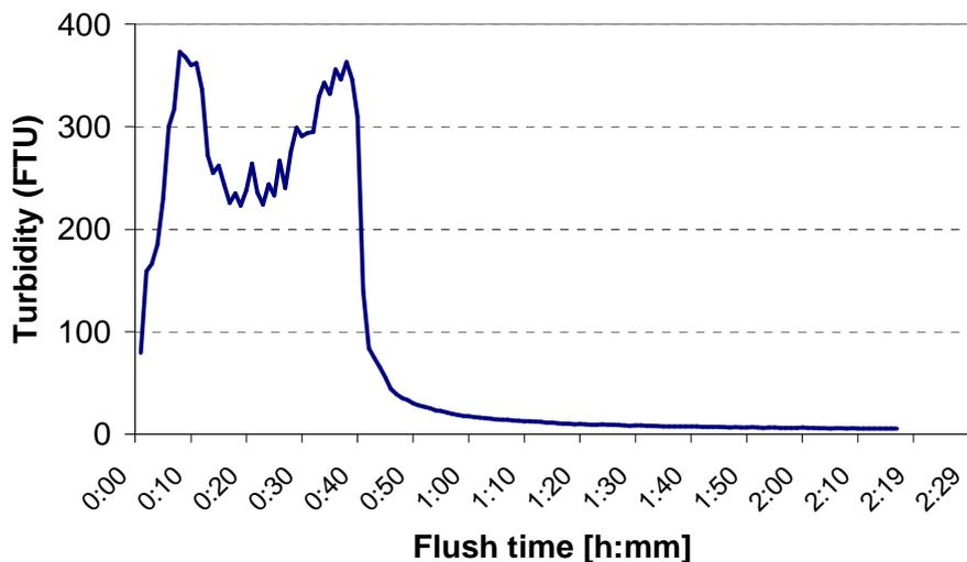
*Fig 5-3 Turbidity measurements at the flushing point of a 300 mm AC pipe, length 3600 m, volume flow 680 m<sup>3</sup>/h (1,5 m/s). Horizontal axis is the time elapsed after the start of the experiment*
