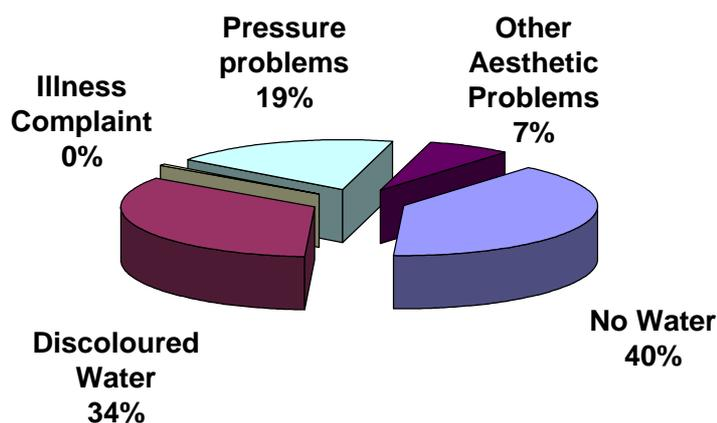
*Fig 1-1 Typical breakdown of reasons for customer contacts for a 5-year period for a UK water company.*
