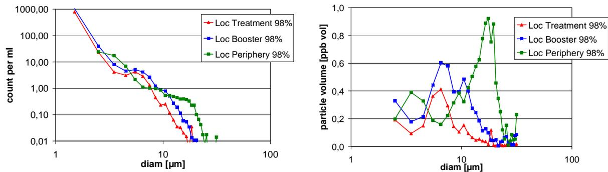
Fig 6-13 Particle size distribution of 98-percentile measurement and volume distribution per diameter range for the three measuring locations
