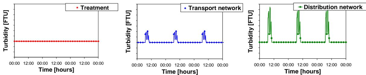
Fig 2-4 Stylistic patterns of turbidity monitoring. Resuspension as result of increased velocity during peak hours. In this case a typical morning peak causes a relatively sharp increase of turbidity. The increase is highest in the distribution network.
