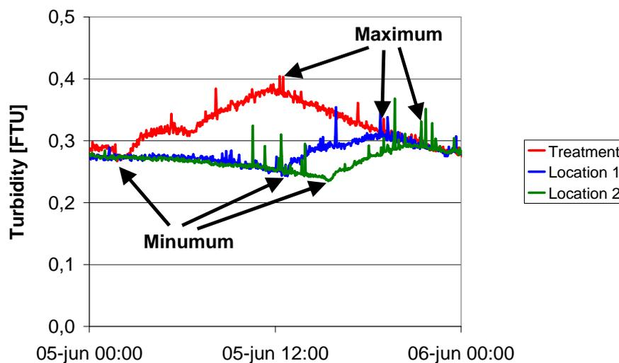
Fig 2-7 Detail of turbidity graph with the maxima and minima indicated
