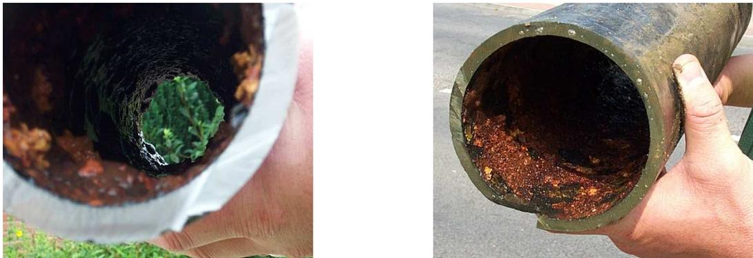
Fig 1-4 Material accumulation around the complete perimeter of cast iron pipe samples
