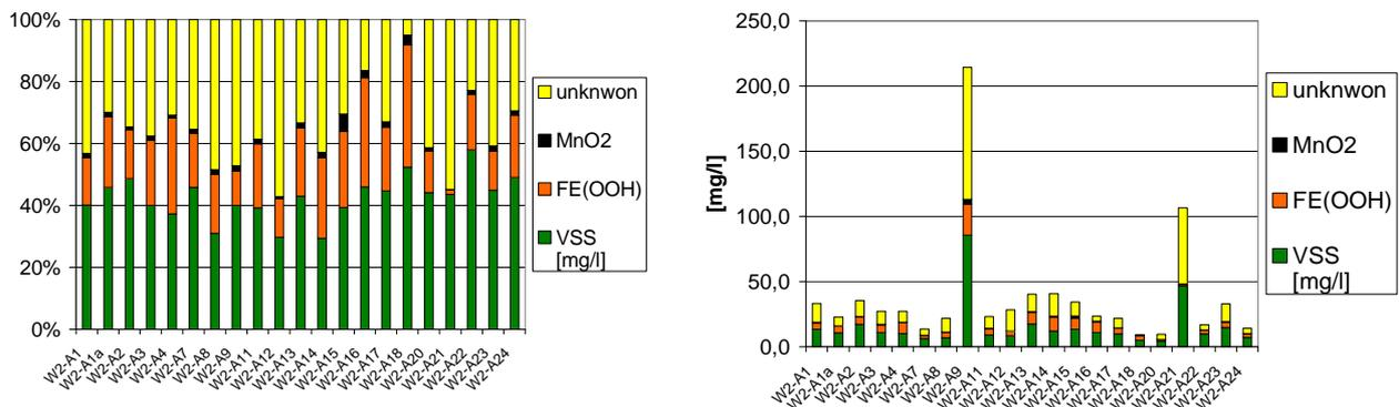
Fig 3-20 Composition of flush samples from Reference Area
