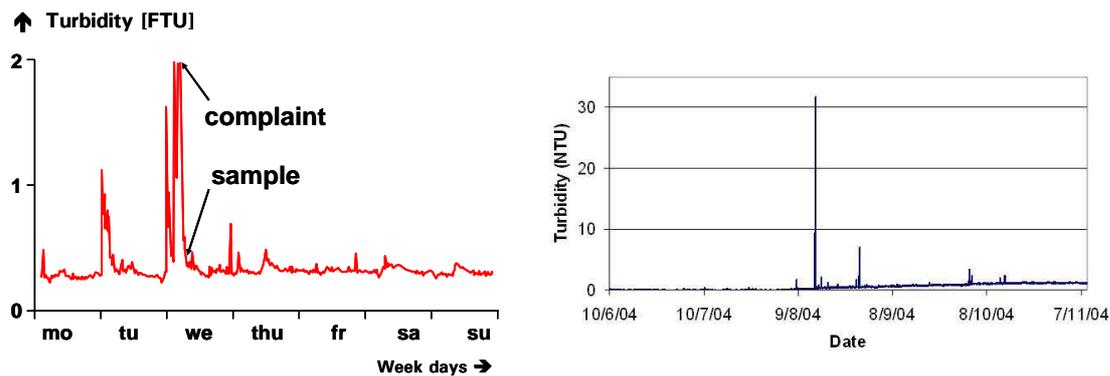
Fig 1-3 Typical discolouration events; both graphs record the turbidity response on a disturbed flow velocity. Left measured in the Netherlands, right a similar incident in the UK (Vreeburg, Boxall 2007)
