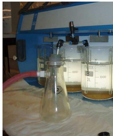
Fig 6-15 Siphon in jar test equipment
