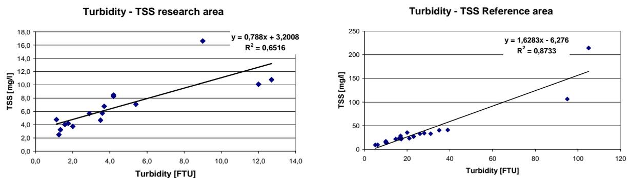
Fig 3-16 Relation Turbidity – TSS for in samples of the flushed water
