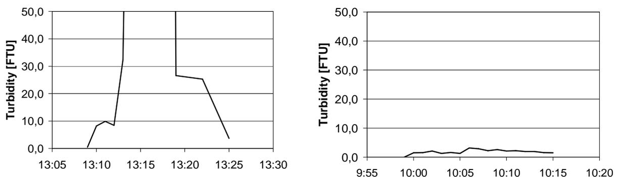
*Fig 2-17 Results of RPM method applied pre- and post-cleaning to evaluate the effectiveness of the operations. The pre-cleaning RPM is 11 according to Table 2-5 and post-cleaning is 1; resettling time is ignored*
