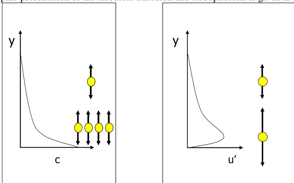
Fig 4-2 Turbulent diffusion (left) and turbophoresis (right)
