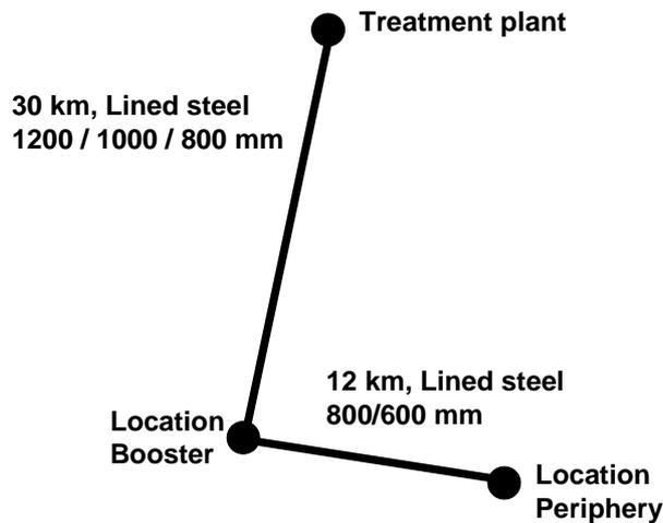
Fig 6-8 Schematic presentation of the monitoring locations
