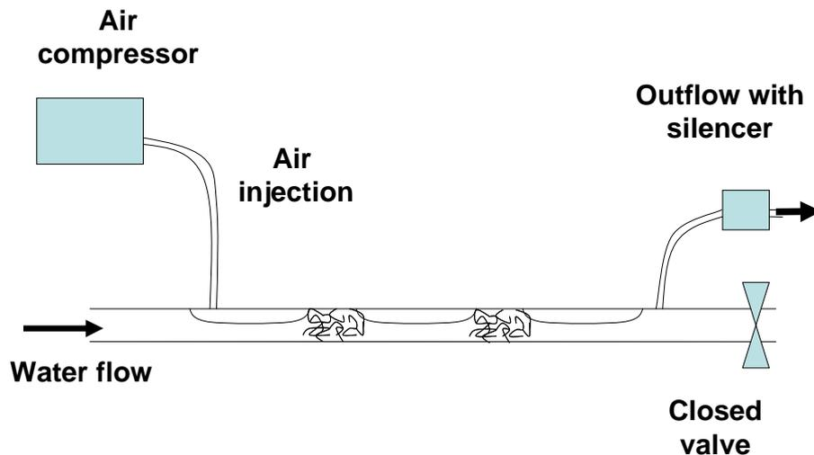
Fig 5-4 Principle of water/air scouring
