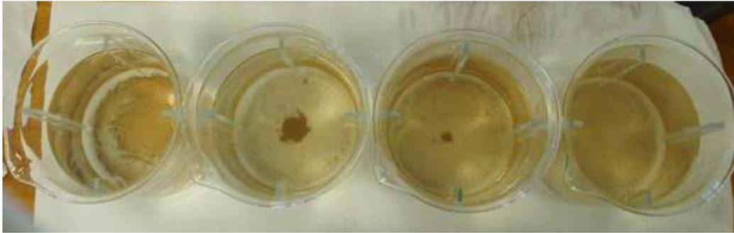
*Fig 6-16 Bottom view Amsterdam C after 10, 30, 60 and 90 RPM*
