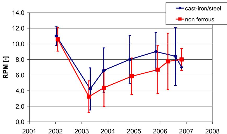
*Fig 5-14 Average RPM's, separated into ferrous and non-ferrous pipe materials; error bars set at one standard deviation*
