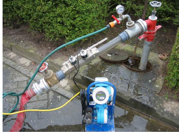
Fig 5-10 Measurement equipment for RPM
