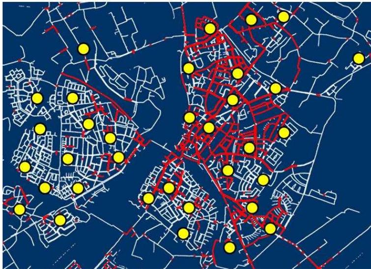
*Fig 5-9 Network in the city of Venlo. The red lines are cast iron or steel, the blue lines are pipes made of non-ferrous material, primarily asbestos cement. The yellow circles represent the RPM-locations.*
