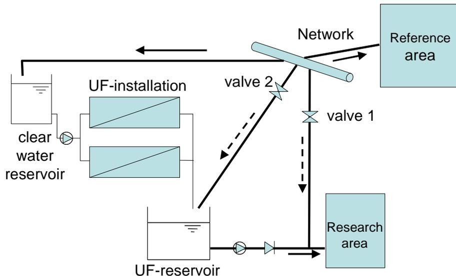
*Fig 3-1 Scheme of UF-installation connection. Valve 1 is controlled by the pressure in the Research Area, valve 2 is controlled by the level in the UF-reservoir. The solid arrows indicate the normal flow direction, the dashed arrows the flow in case of failure of the UF-installation or the pump*
