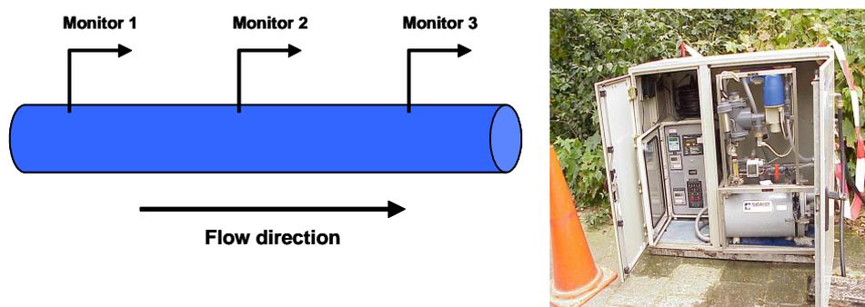
*Fig 2-2 Schematic of monitoring with continuous monitoring equipment and a picture of a mobile system.*
