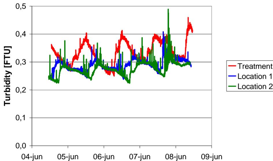
*Fig 2-6 Example of continuous monitoring of turbidity at the treatment and two locations in the network. The variation in turbidity at the treatment plant is mirrored in the network, showing a general decrease of the values of turbidity.*
