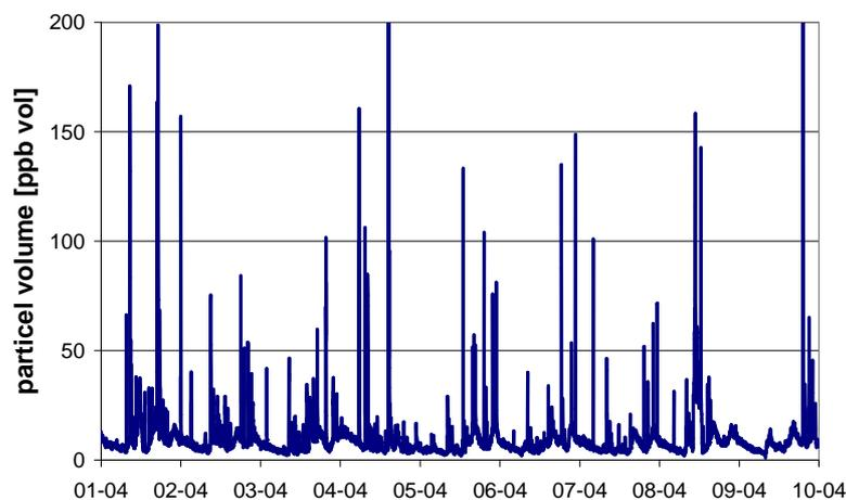
*Fig 2-10 Calculated particle volume during a period 9 days of measuring with a 2 minutes sampling frequency*
