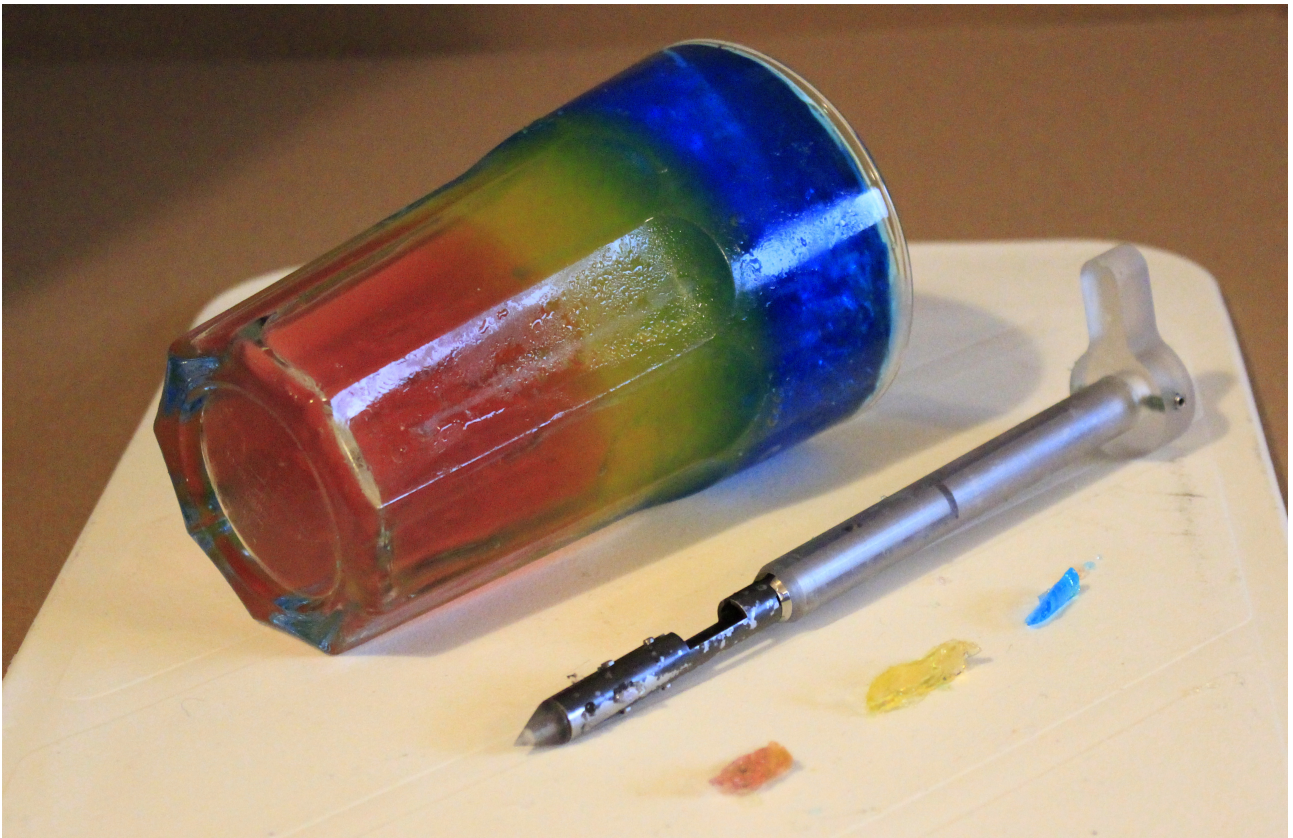
Figure 4.2: The result of the biopsy transport experiment. Visible is the glass with the multicolored gelatin, the biopsy needle and the three differently colored pieces of gelatin, extracted from the glass using the biopsy needle.
