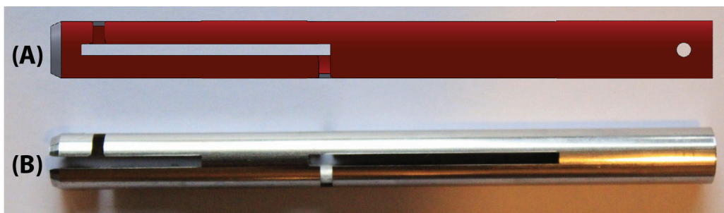
Figure 3.6: Side view of the bayonet needle of the prototype. (A) shows the sideview of the design of the simplified bayonet needle for the final prototype. The cut-outs at the tip have been simplified due to the elongated barriers from figure 3.3. (B) shows the stainless steel tube that has been manufactured for the final prototype.
