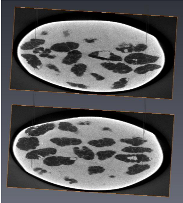
Figure 15 CT image of the two coco pop layers after loading. The scale is given by the sample diameter (55 mm).
