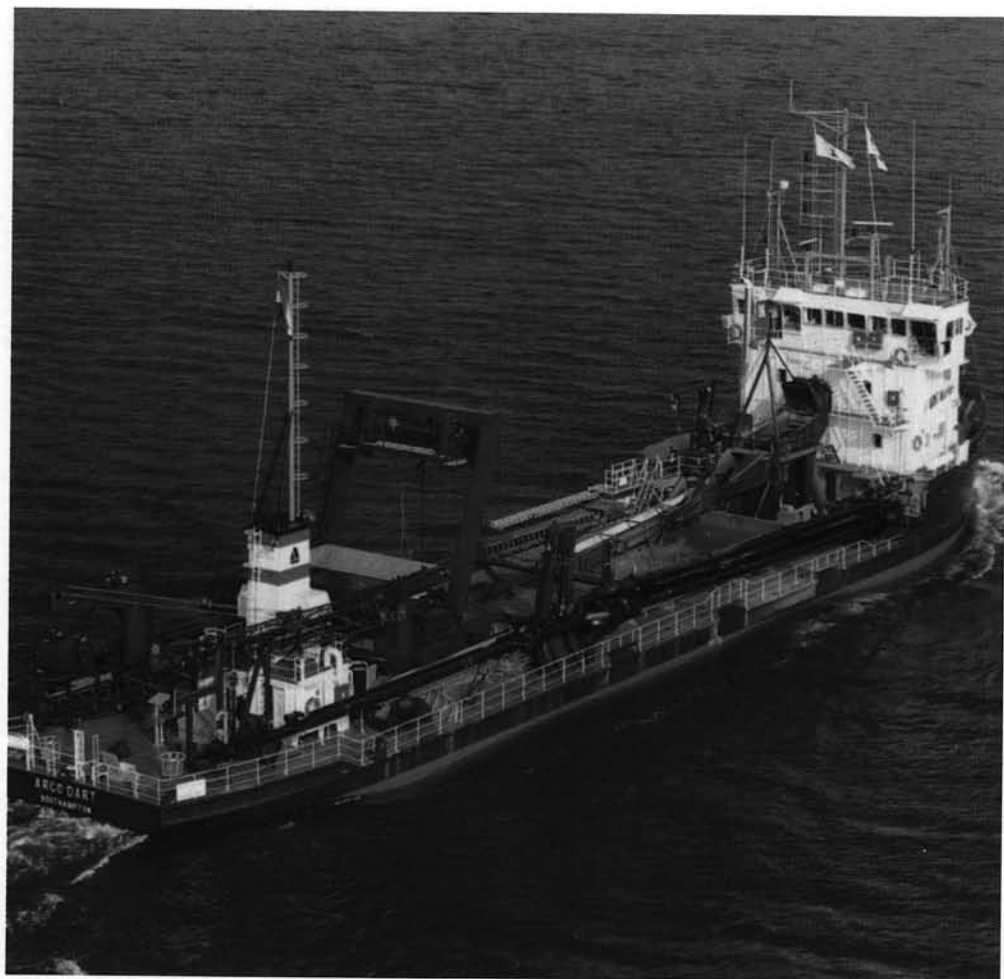
Gravel dredger Arco Dart, with ancilliary equipment such as gravel screens and crane for discharging.
