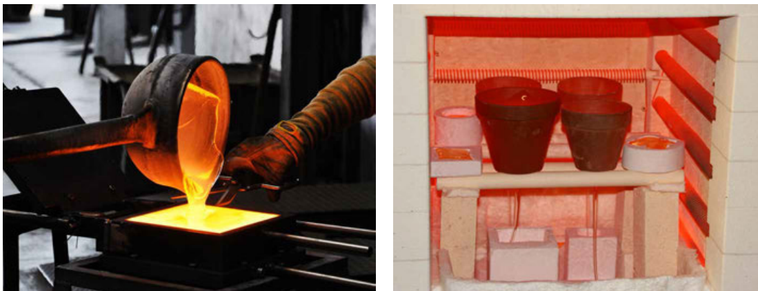
Figure 10: Left: Hot-forming as primary casting process. Right: Kiln-casting as secondary casting process. Retrieved from (Oikonomopoulou, 2019).
