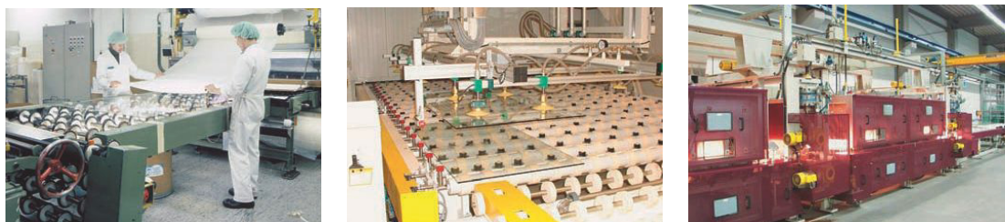
Figure 80: From left to right: PVB film is positioning, placement of the next glass layer on top, pre-lamination. Retrieved from (Wurm,2007).
