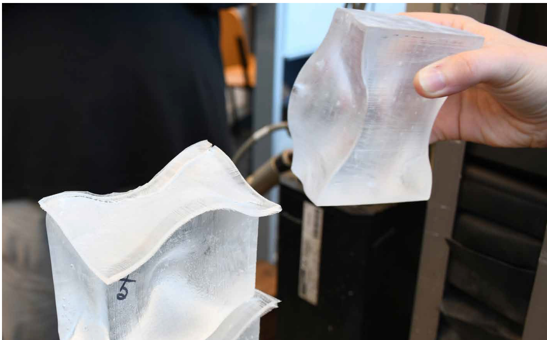
Figure 22: 3 mm thick, cast interlayer from PU70 prototype (Oikonomopoulou et al. 2018).
