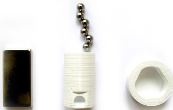
Figure 72: The 3D-printed mock - up, a neodymium magnet and stainless-steel balls assisted to the decision of the final design.
