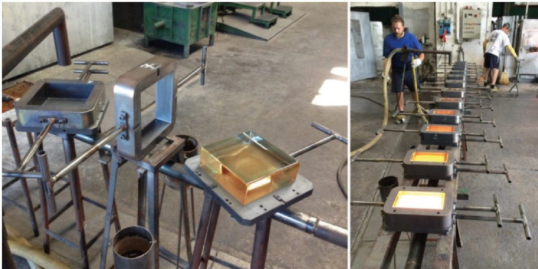
Figure 13: Permanent open steel moulds of high precision designed for the manufacturing of the glass bricks for the Crystal Houses. Retrieved from (Oikonomoulou F. et al., 2018).
