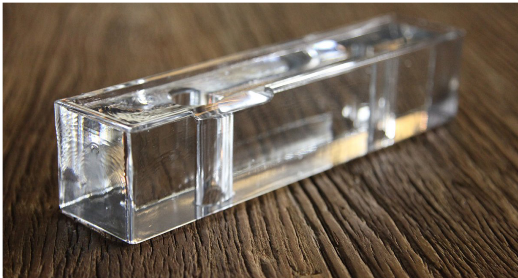
Figure 30: Cast glass brick of the Optical House. Source: HIROSHI NAKAMURA & NAP.
