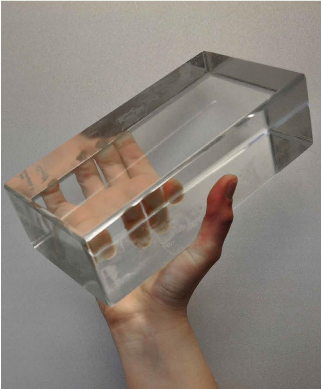
Figure 2: The cast glass unit manufactured by soda- lime glass employed in the Crystal Houses . Retrieved from (Oikonomopoulou, 2019).
