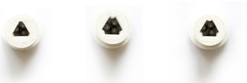
Figure 68: Left: Photo of the first alternative 30°-40°-50°. Middle: Photo of the second and selected alternative with the 40°-45°-50°. Right: Photo of the third alternative with the same inclinations in the inner section.
