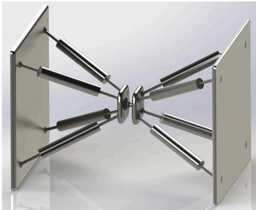
Figure 6, Combination model representing a hinged joint between two floating modules [63].
