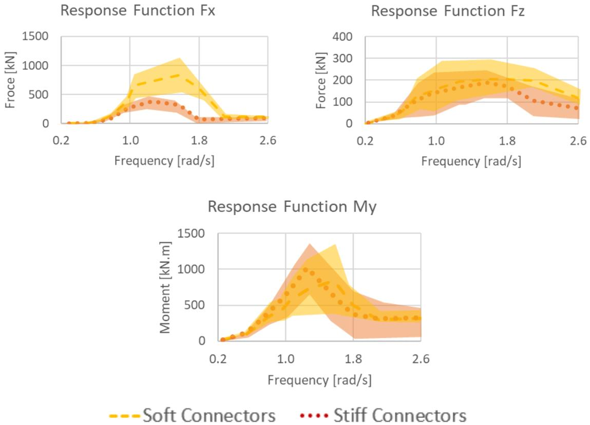
Figure 47, Frequency response functions for averaged  $F_x$ ,  $F_z$ ,  $M_y$  at the connector of the grid model. Results shown for soft (dashed line) and stiff (dotted line) connector stiffness. Shaded zones represent the minimum and maximum values.
