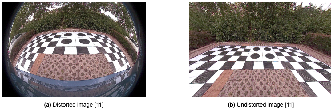
Figure 4.4: Undistortion using OpenCV
