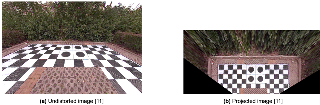
Figure 4.8: Top-down view projection for manual extrinsic calibration using OpenCV
