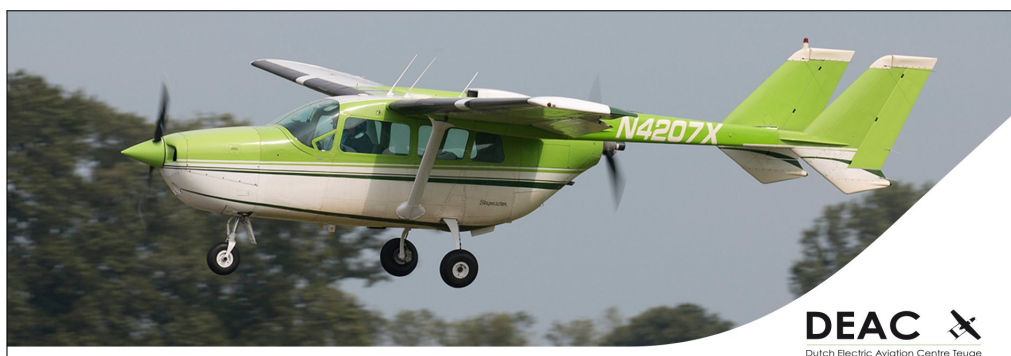
Figure 1.1: The Cessna Skymaster 337F being used as an experimental flying testbed by the Dutch Electric Aviation Centre [9]. Image credits and source: DEAC website.
