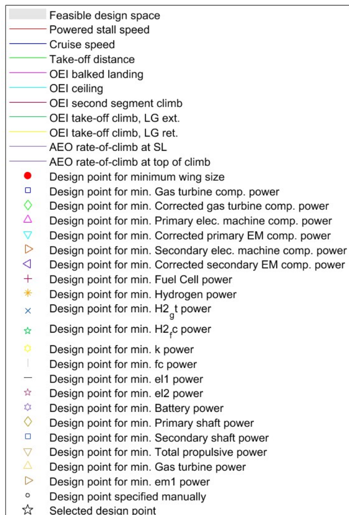
Figure B.1: Legend for the constraint curves and design points used WP/WS sizing diagrams
