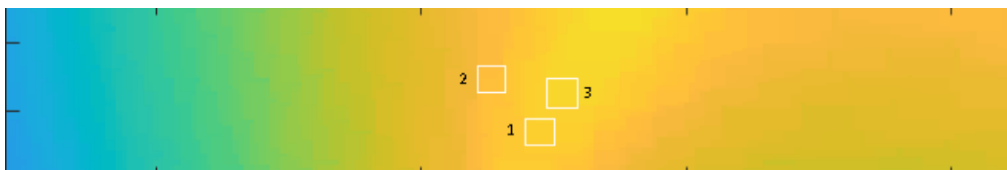
Figure 6.7: Magnified view of post pixel binning with three sample pixel blocks marked. Pixels 1, 2, and 3 roughly fall within the same pixel intensity, and the ability to distinguish between their values is integral to the processing algorithm.
