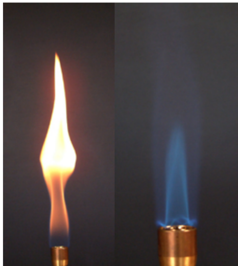
Figure 4.2: Visual differences between a premixed shown on the right and an example of a diffusion flame shown on the left. Note the characteristic difference in the color of the flame which is a direct result of the manner in which the reactants interact with one another during combustion
