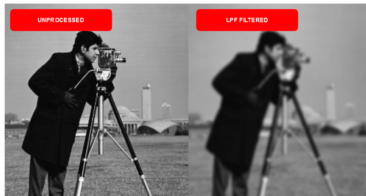
Figure 6.15: Effect of applying low-pass filters on an example image. Comparing the unprocessed image on the left, the sharpness of the image has been reduced and an overall blurring effect has been produced.
