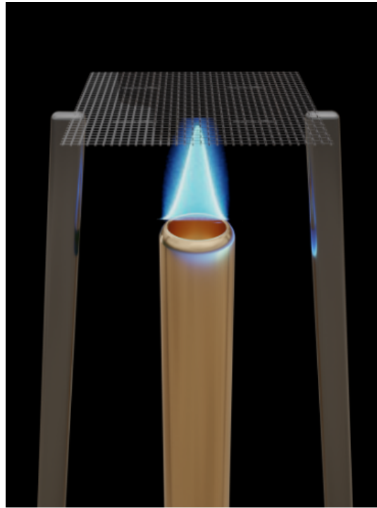
Figure 9.1: Schematic representation of wire mesh placement over the conical flame burner. Note the simple construction and the possibility of varying the position of the mesh with varying flame configurations as needed.
