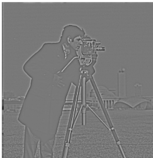
Figure 6.10: High pass filtered image (processed). The highlighted regions (white) of the image show the sharp edges that are present in the image - [43]
