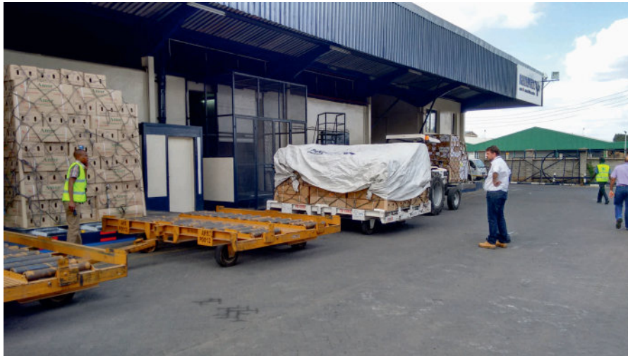
Figure 6.4: A build up pallet with an insulating cover
