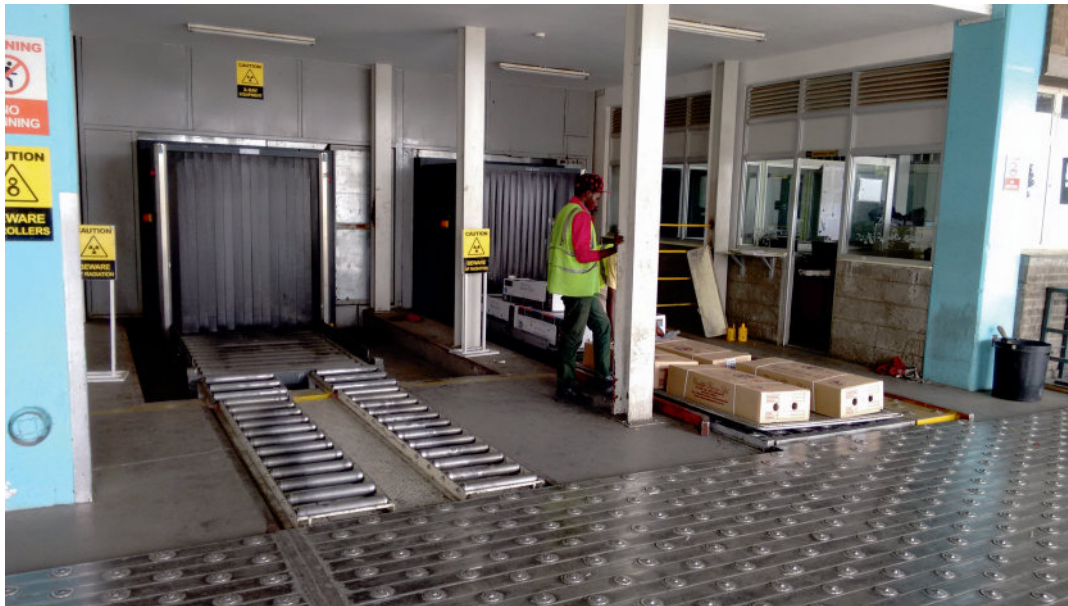
Figure B.19: Acceptance area for loose cargo with X-ray scanners in the back
