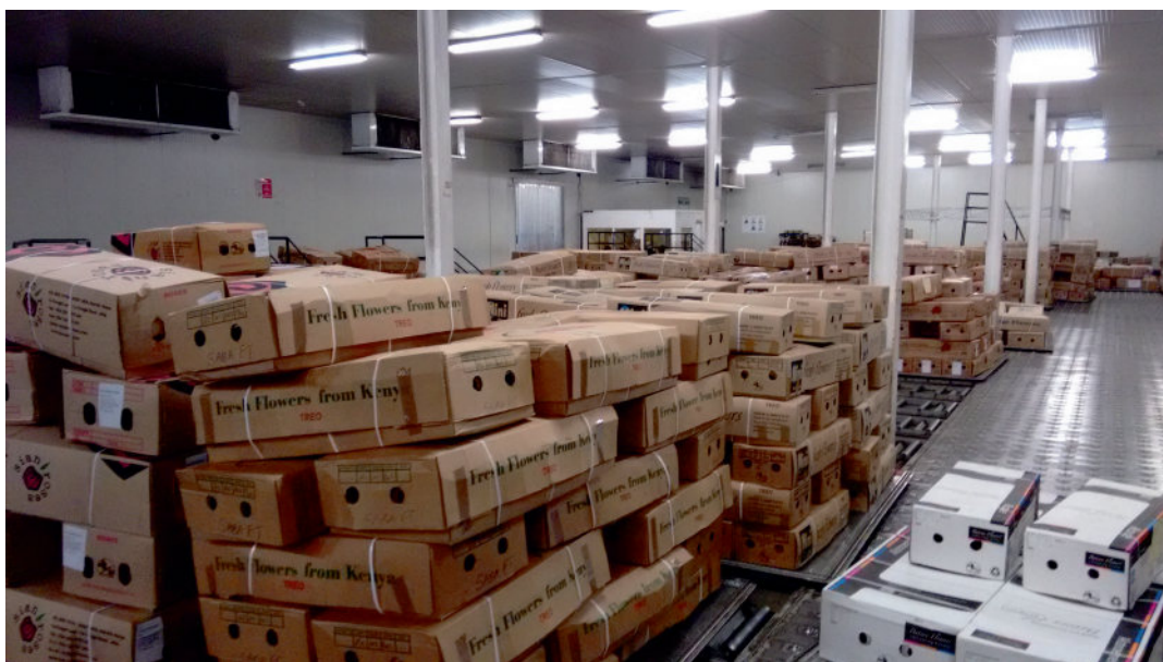
Figure B.20: First cool room where boxes are stapled in such a way to create funnels
