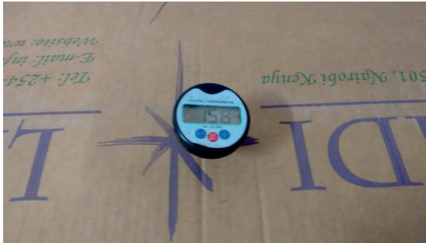
Figure 5.6: Temperature sensor showing measured temperature of a box
