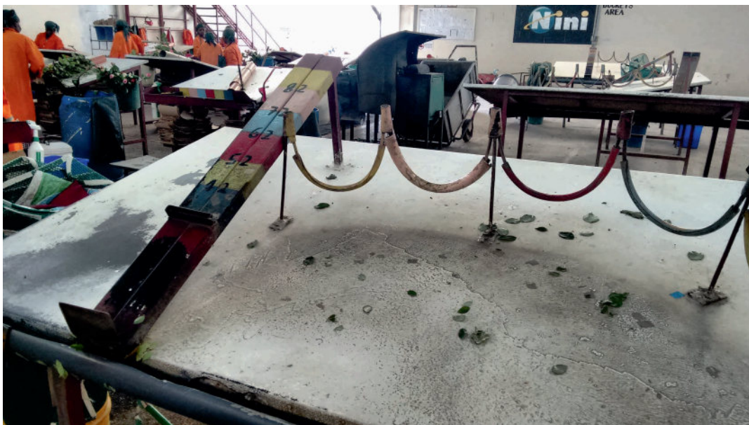
Figure B.3: Table where rose is graded, ruler at the left indicates stem length
