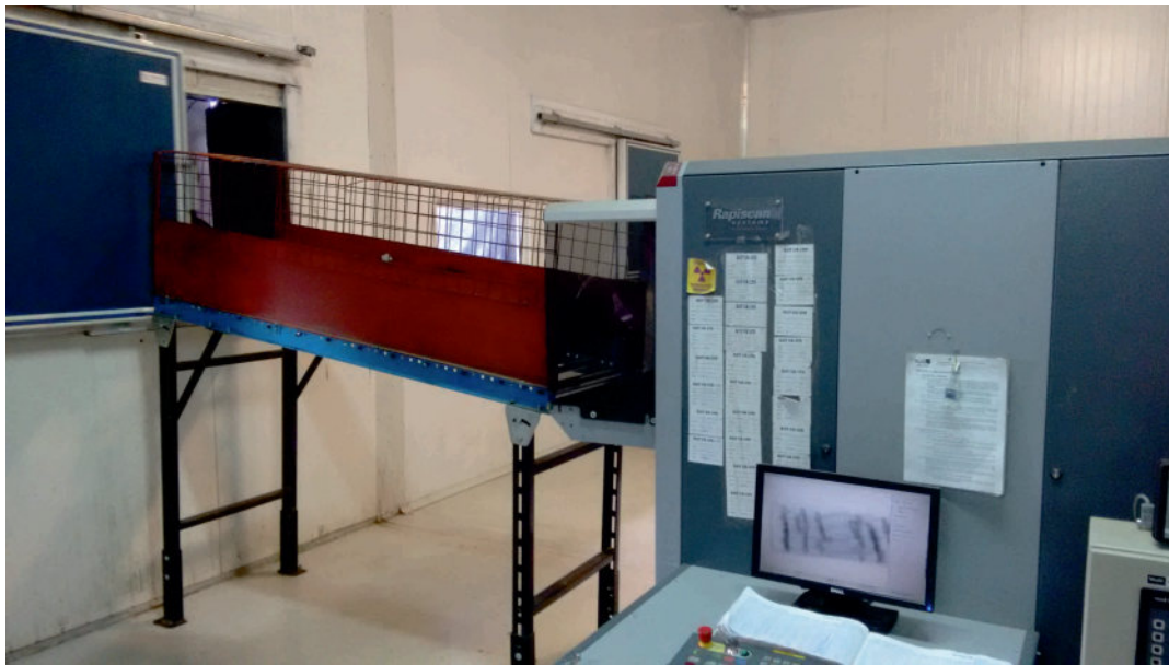
Figure B.8: X-Ray scanner checking incoming boxes
