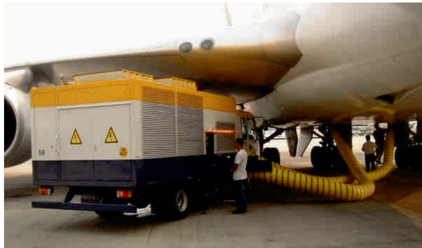
Figure 6.6: Example of an air conditioning unit pre-cooling the aircraft
