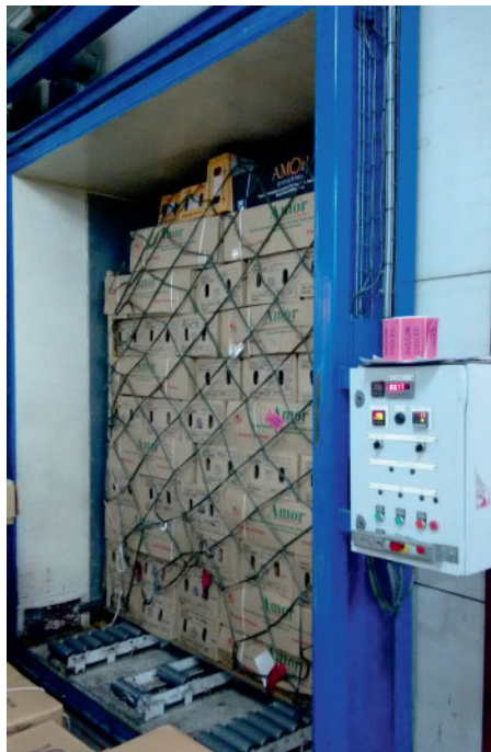
(a) An aircraft pallet ready to be vacuum cooled
