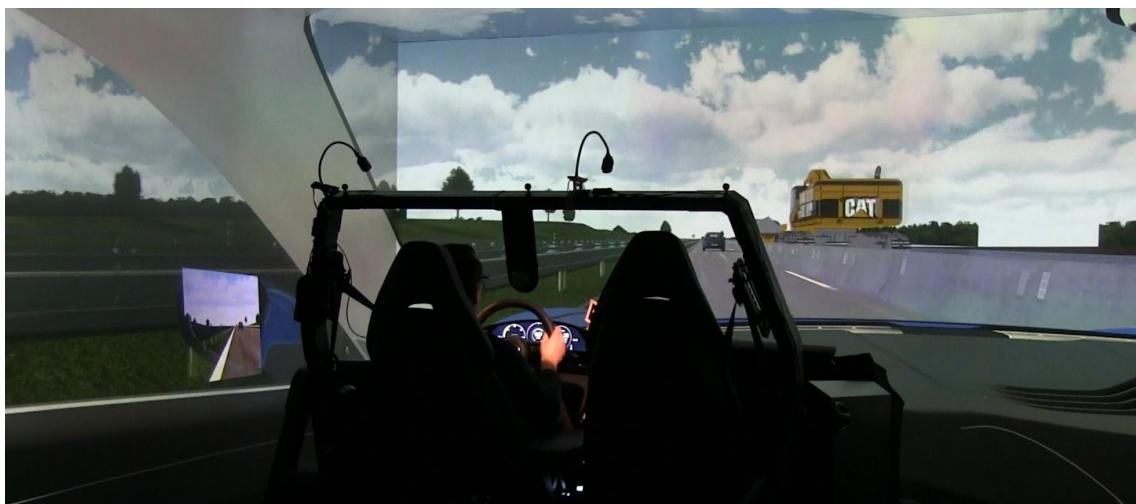
Figure 2.3: The hexapod simulator during take-over scenario 1. The participant has regained manual control and executed an emergency lane change to the left lane. Roadworks can be seen projected on the right lane.
