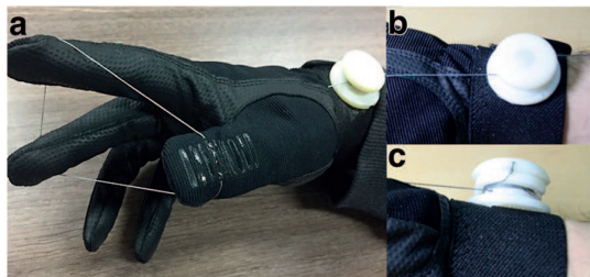
(a) Overview working mechanism GRIPIT (Kim et al., 2017). The wire is the part that makes it able to grip something.
