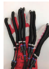
(i) Design of AI Fahaam hand orthosis (AI-Fahaam et al., 2018). In this situation is the PAM placed on top of the fingers.
