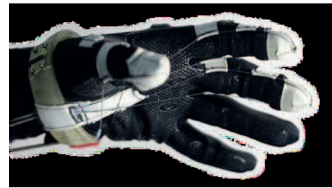
(j) Overview EXO-Glove soft wearable hand orthosis with the integrated working mechanism (Jeong et al., 2015).
