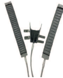
(e) The pneumatic actuators of Jiralerspong for the fingers and the thumb (Jiralerspong et al., 2018).
